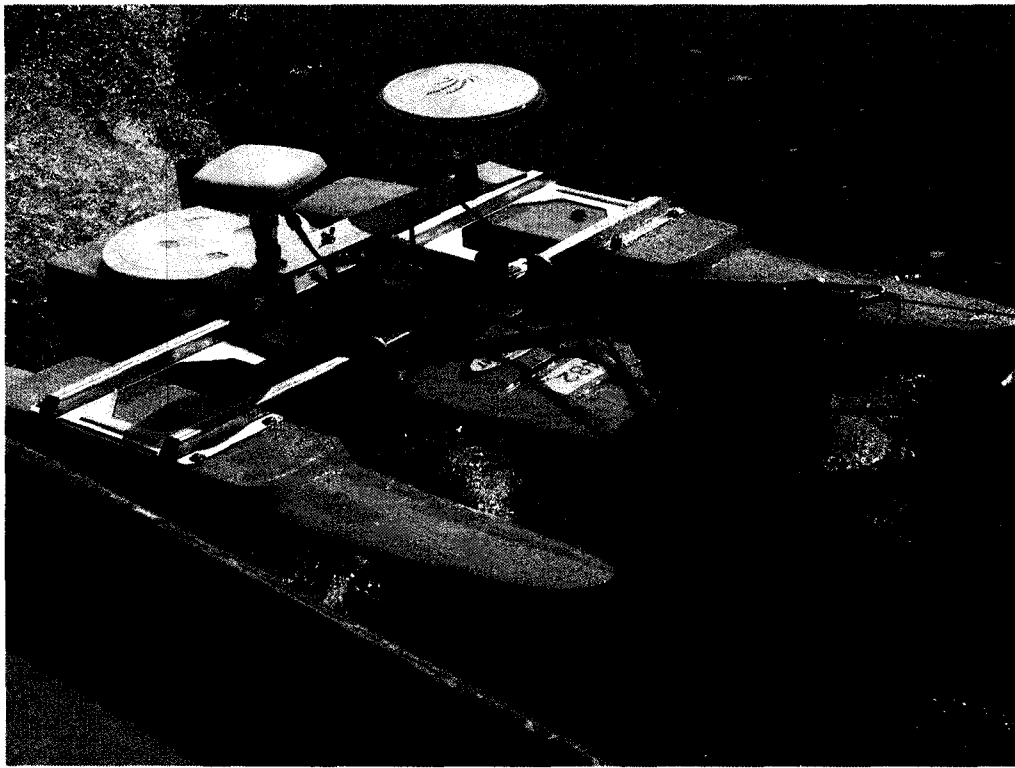
Figure 5.2 Set up of aDcp and NovAtel receivers at Bow River, Alberta.
