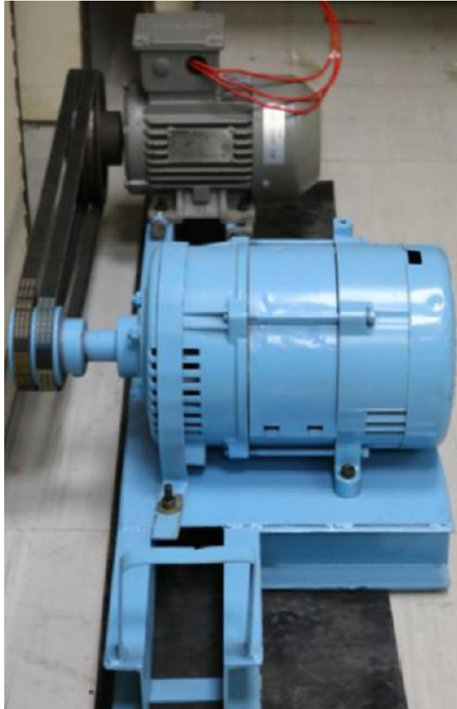
Figure 3-2. Triaxial Bearing Data Test Rig [27]
