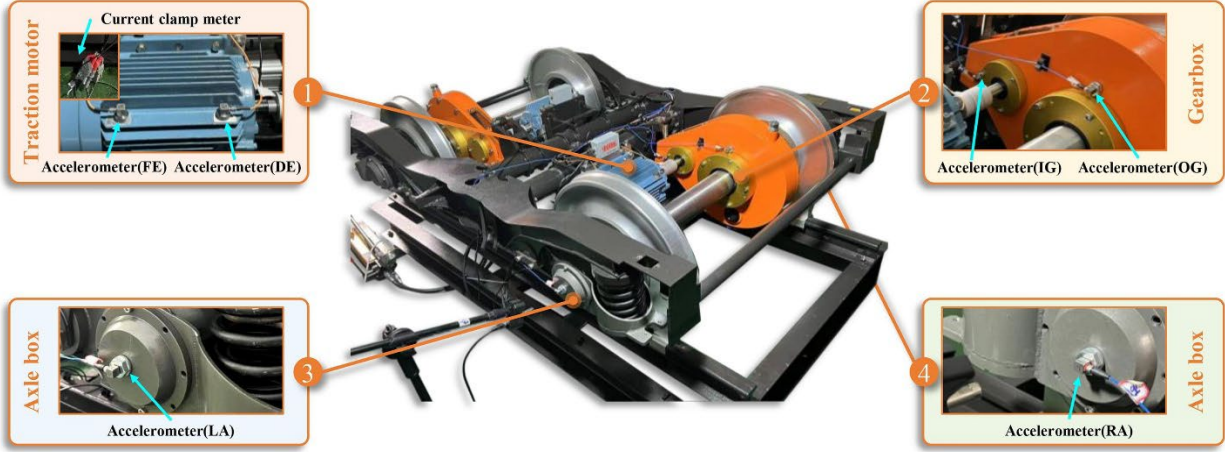
Figure 3-5. IEEE PHM Beijing 2024 Data Challenge Test Rig Setup [35]
