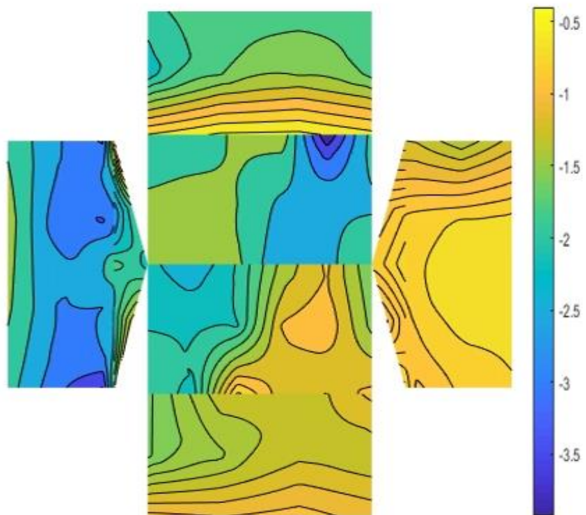
Figure A.10: Model 2, Case 7 (BOA:0°, D:40cm) Peak pressure coefficient contour plot
