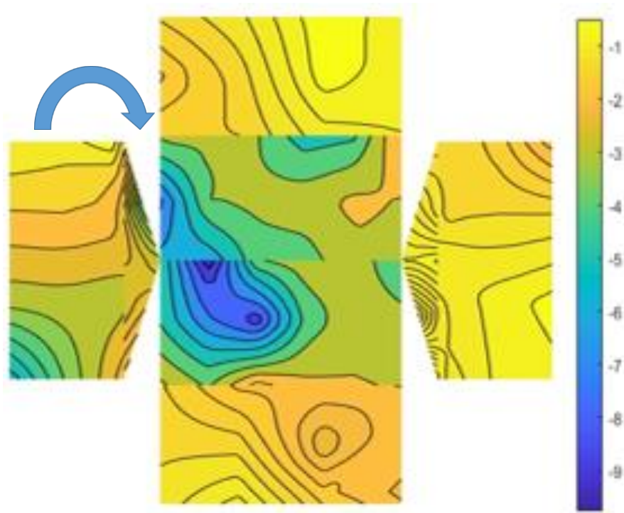
Figure 4.7: Model 2, Case 1 (BOA: 0^\circ , D: 10cm) Peak pressure coefficient contour plot
