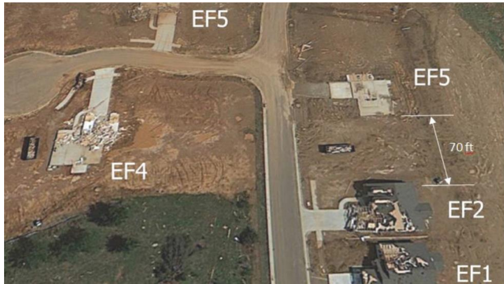
Figure 1.1: Aerial image of different EF scale tornadoes aftermath (Ramseyer et al., 2015)
