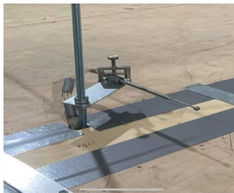
Figure 3.2: Omniprobe sensor used to determine velocity parameters of experimental vortex
