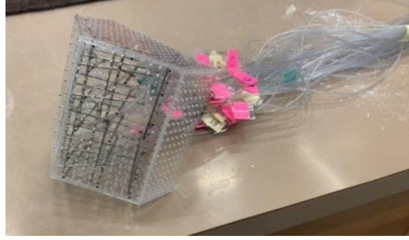
Figure 3.6: Pressure taps installed on the roof of the model for phase 2 experiments
