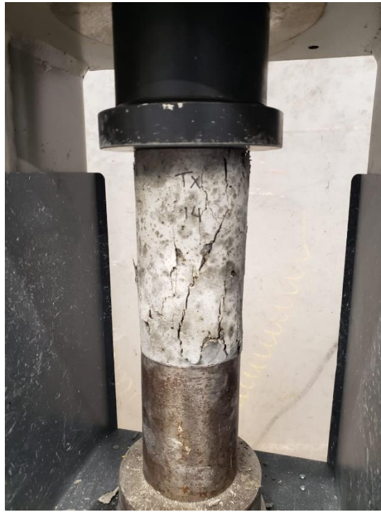
Figure 27: Mechanical analyses – A and B) SDT and C) Compressive strength.
