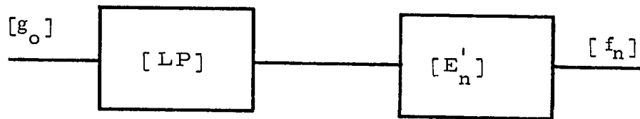
Fig. 4.4.b Reduction of the iterative extrapolation process to two matrix operations
