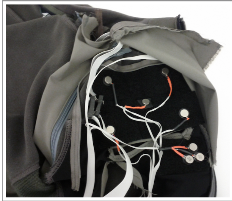
Figure 4.12 Inside the left side chest area showing 3 vibrotactile actuators for the heartbeats
