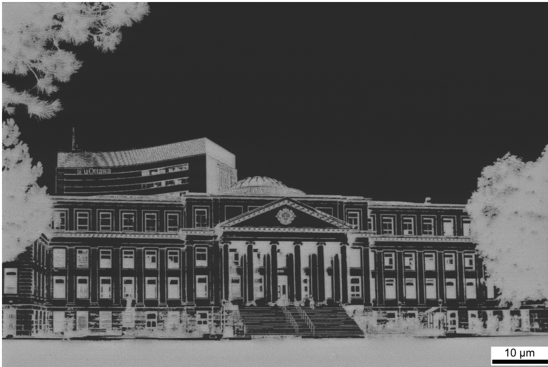
Figure S2. HIM image of Tabaret Hall (with Desmarais Hall in the background) at the University of Ottawa, patterned in PMMA on a silicon substrate, then developed. A helium ion beam current of 1.5 pA was used to deliver a dose of 8 \mu\text{C}/\text{cm}^2 . Dark grey is PMMA and light grey is silicon. Sub-20 nm features are resolved on this pattern. A write-field of 150 \mu\text{m} was used to define the image. (Photograph courtesy of Bonnie Findley, University of Ottawa.)
