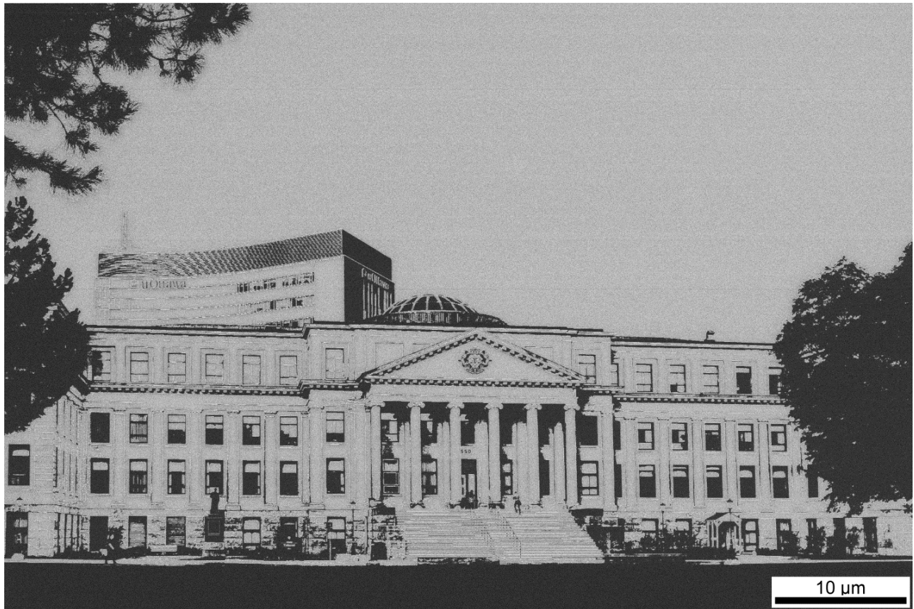
Figure 3.2.3. HIM image of Tabaret Hall at the University of Ottawa on Si. Dark regions are crosslinked PMMA whereas the substrate is seen on the light regions. Photograph courtesy of Bonnie Findley (University of Ottawa).
