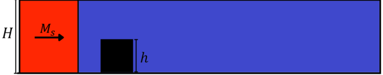
Figure 3.1: Schematic of the computational domain. A planar shock of Mach number M_s propagates through a channel of height H toward a square obstacle of height h = 0.4H placed at the bottom wall.
