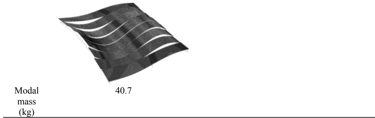
Fig. 5.5. Effect of boundary conditions on vibration modes of a 5m by 5m floor with three beams
