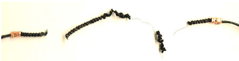
Figure 4-1 Overheated polyethylene TCP actuator failure in numerous locations
