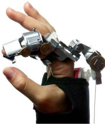
Figure 2-5 HANDEXOS - individual finger module [33]
