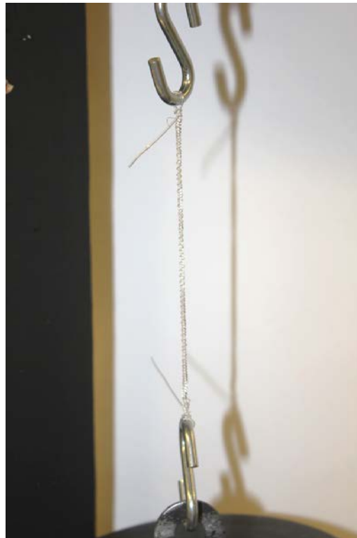
Figure 3-7 Big Game fishing line twisted and coiled with a manually wrapped Koiler resistance wire
