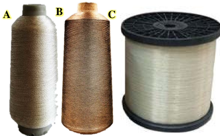
Figure 3-1 Tested Nylon fibres: (A) Shieldex conductive nylon fibre 117/17, (B) Shieldex conductive nylon fibre 235/34, and (C) 10lb nylon 6 monofilament fishing line
