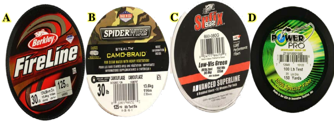
Figure 3-2 Polyethylene test fibres (A) Berkley FireLine 30lb test line, (B) SPIDERWIRE camo-braid 30lb test line, (C) Sufix 832 Low-Vis 80lb test line, and (D) PowerPro braided 100lb test line
