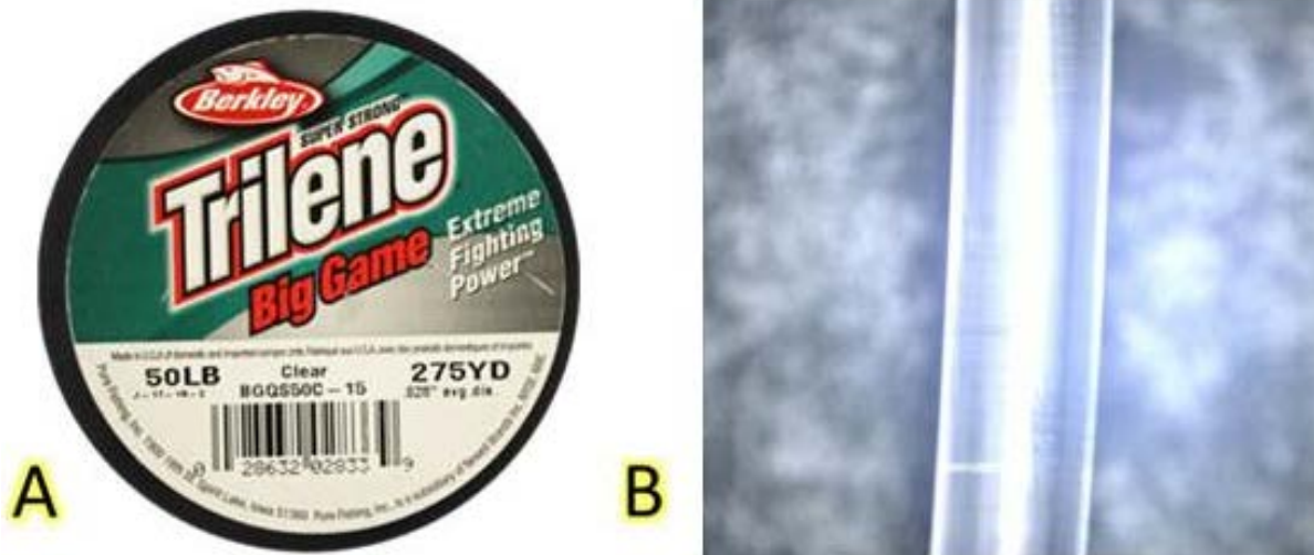
Figure 3-3 (A) Trilene Big Game 50lb test line (B) 100x optical magnification of this fibre 770 µm
