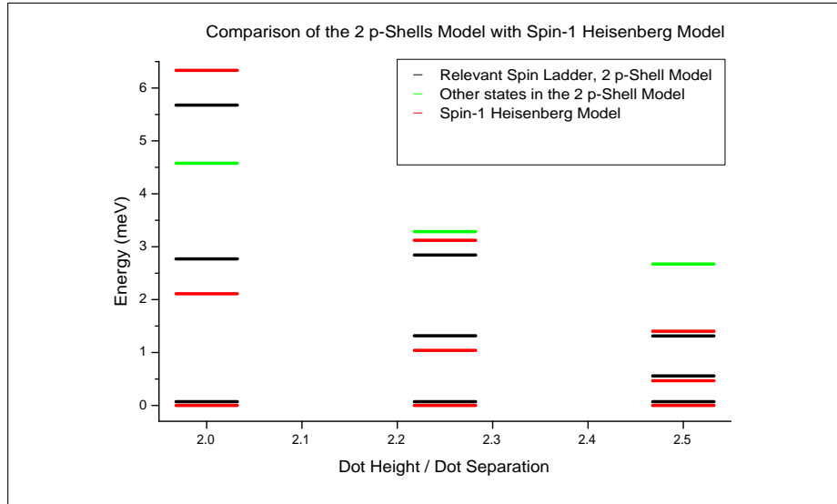
Figure 3.5: Comparison between the CI treatment of 4 electrons on 2 p -shells and the Heisenberg spin model for different dot separations. Degeneracy is not resolved. The black levels are L = 0 levels from CI; they are from lowest in energy to highest: the spin singlet, triplet, and quintuplet. The green levels are other levels from the CI spectrum. The Heisenberg J was fitted in the same manner as in Figure 3.4b.
