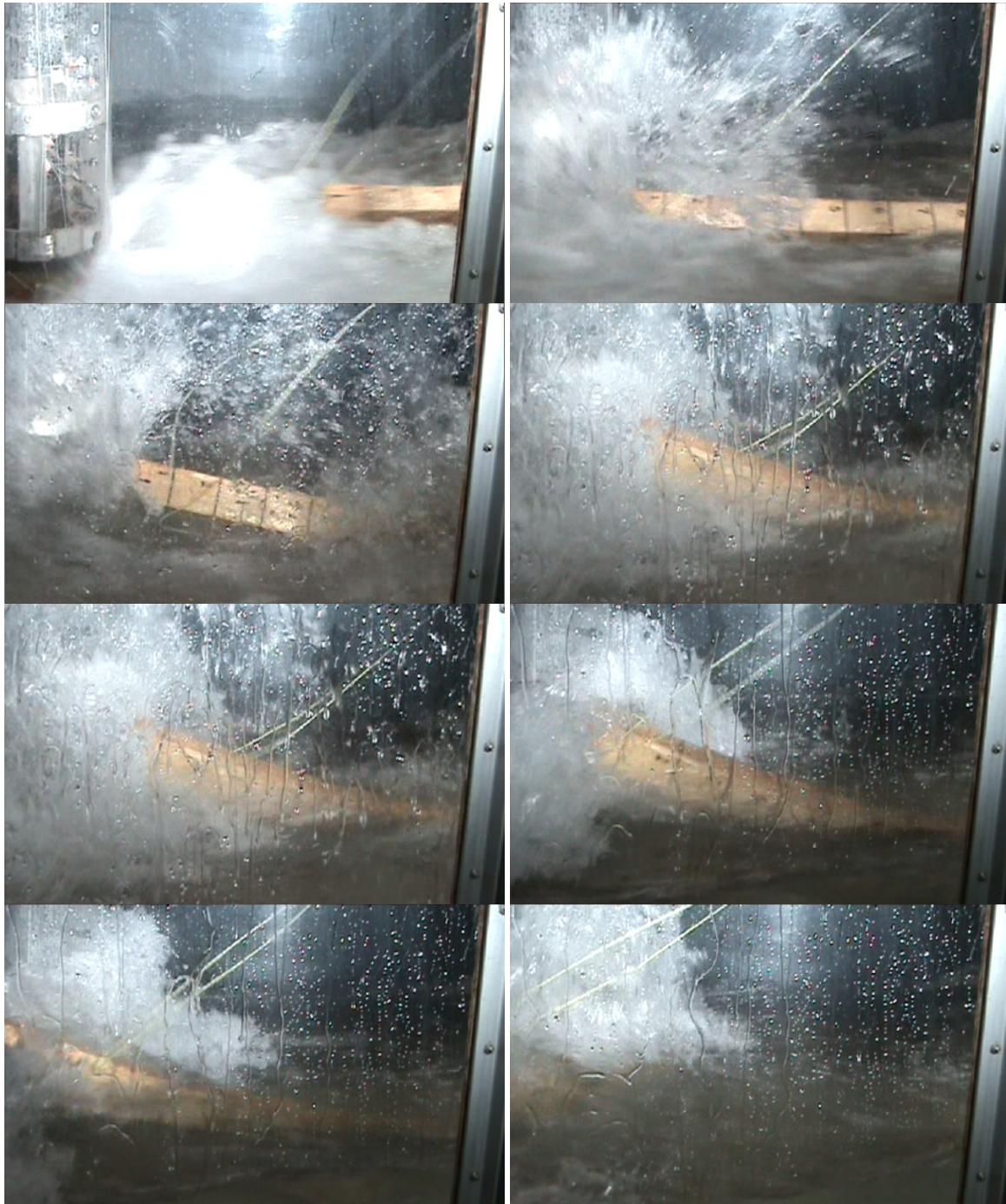
Figure C-6. Photos for 2kg1P debris floating in hydraulic bore generated from 850 mm impounding depth: side view
