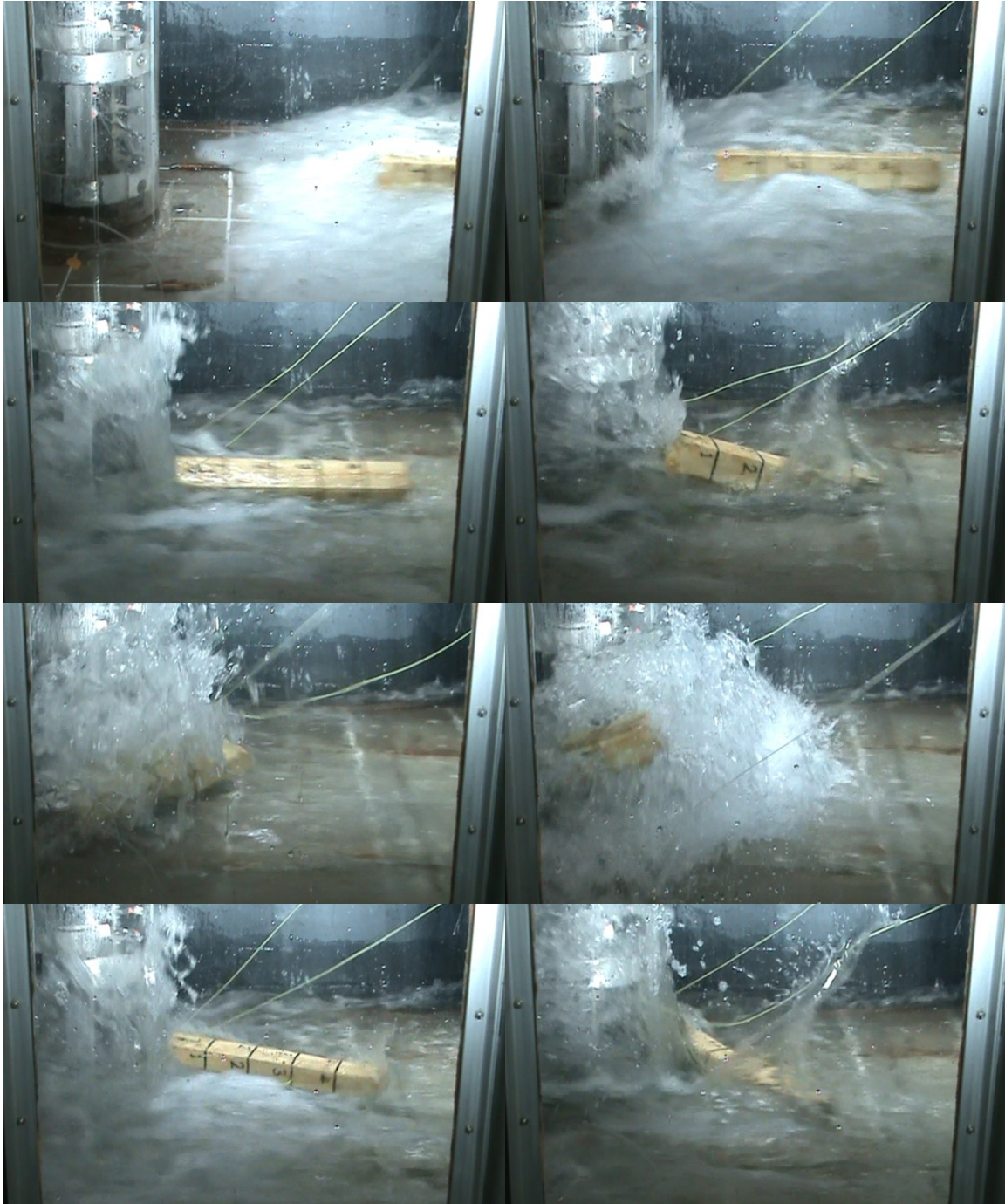
Figure C-4. Photos for 1kg debris floating in hydraulic bore generated from 550 mm impounding depth: side view
