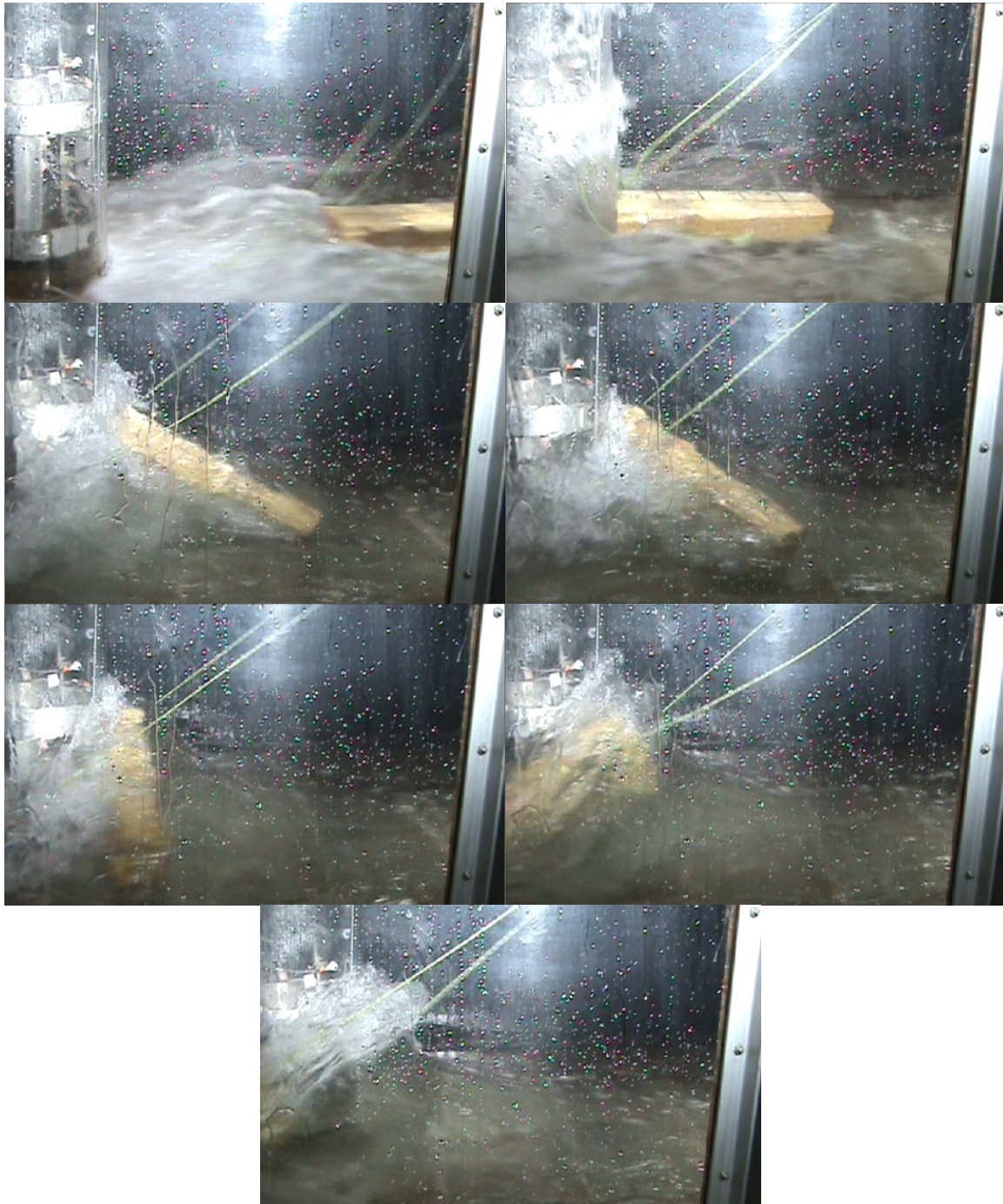
Figure C-8. Photos for 2kg2P debris floating in hydraulic bore generated from 850 mm impounding depth: side view
