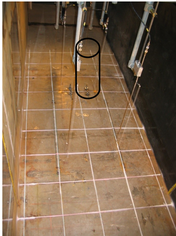
Figure 4.15 Grid spacing of 300 mm x 300 mm marked on the flume bed
