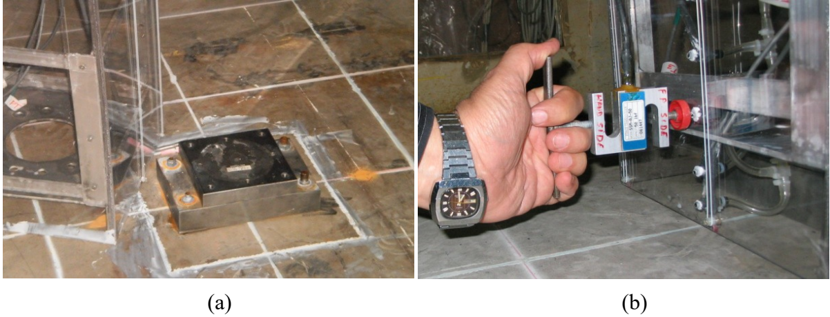
Figure 4.11 Dynamometer and reference load cell: a) dynamometer MC6; and b) reference load cell
