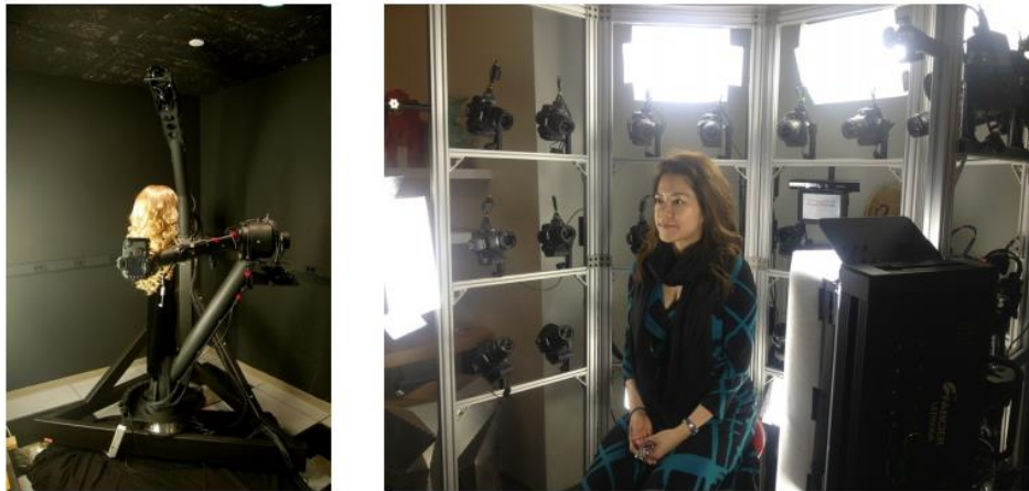
Figure 2.3: The capture system used in “Structure-Aware Hair Capture” method [20] , a robotic gantry and SLR camera to capture images for the wigs (left), a camera array of 30 SLR cameras for real hairstyle (right).
