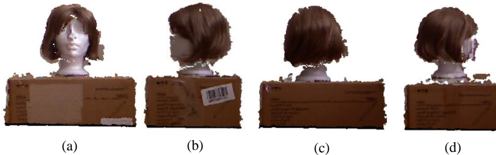
Figure 3.8: Applying same segmentation to the point clouds from the four Kinect sensors.
