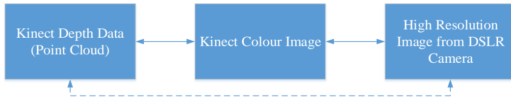
Figure 3.11: Build the correspondence between depth data and high resolution image through the connections of depth data and colour data, and colour data and high resolution image.
