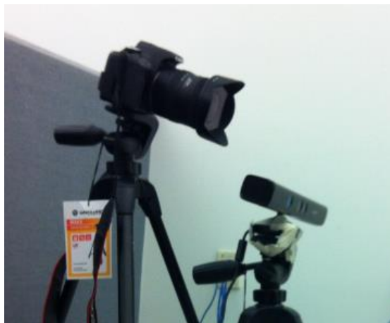
Figure 3.14: The Kinect sensor and DSLR camera used in the experiment.
