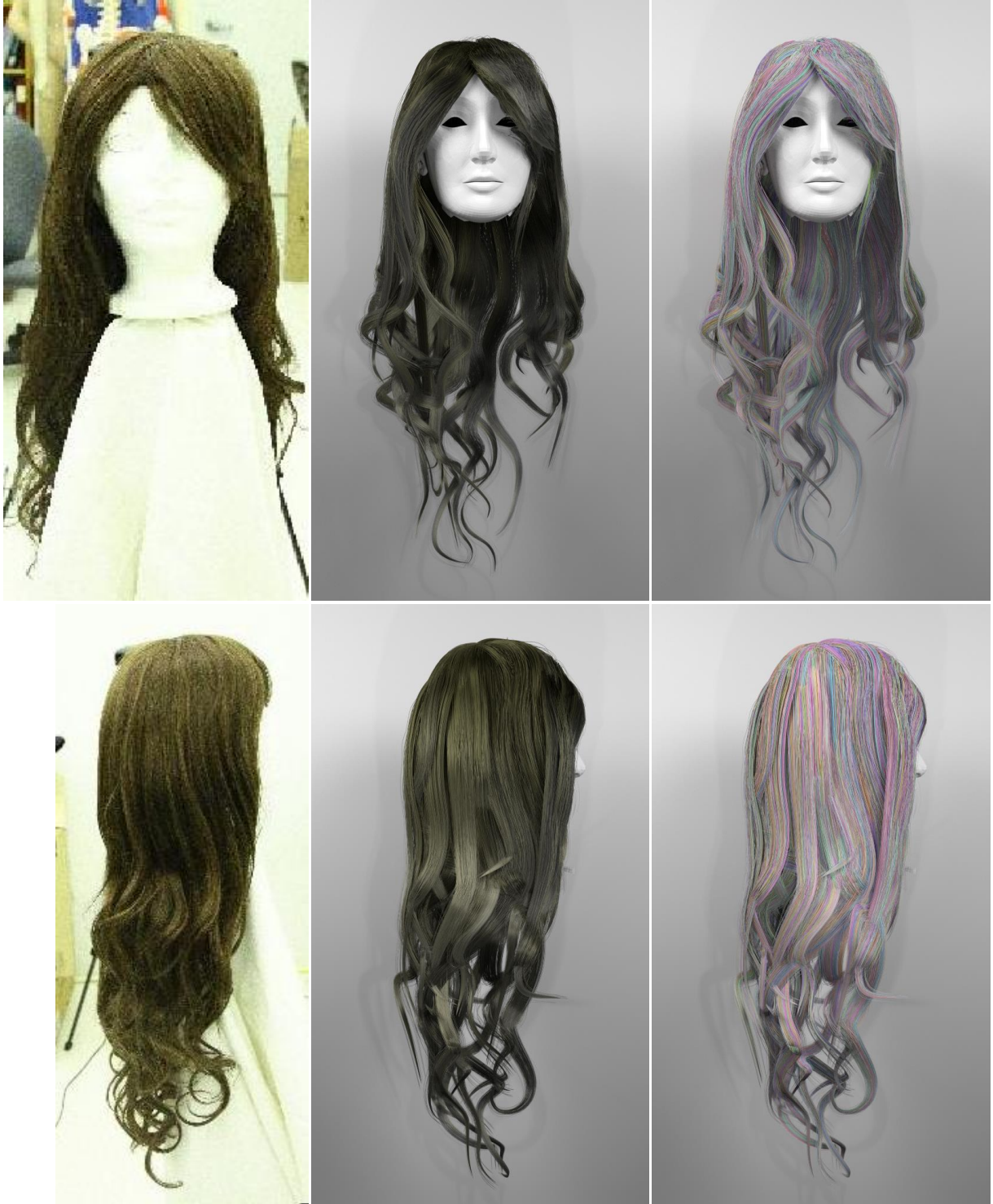
Figure 6.19: The comparisons of the front and left view data set, the left row images are the input high resolution images, the middle row images are the regular rendering results, and the right row images are rendering results with colour-coded hair strand.
