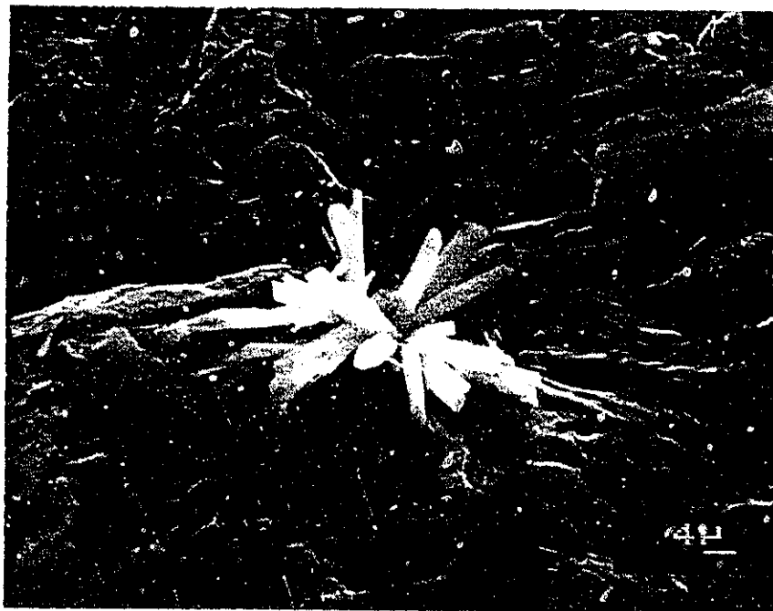
Figure 2.6: SEM micrograph of a cluster of crystals of a bismuth compound on the surface of a graphite rod.
