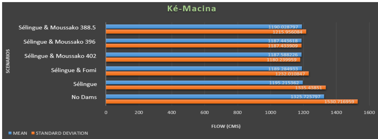
Figure 58: Ké-Macina subwatershed annual flow mean and standard deviation under different scenarios with OdN (2035 Irrigation Scenario).
