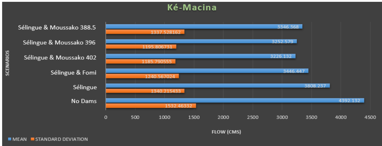
Figure 73: Ké-Macina subwatershed wettest month flow mean and standard deviation under different scenarios, with OdN.
