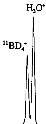
Figure 6.3 High Mass Resolution of m/z 19 in the Normal Mass Spectrum of B 2 D 6
