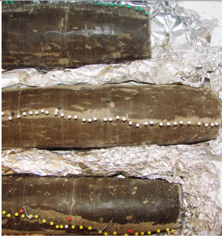
Figure 3.2: Marker beds in all three cores, core 1 (top), core 2 (middle), core 3 (bottom). The bottom of the core is to the right, and the pins denote 10-year sections of the core, photo no. DSC09945.
