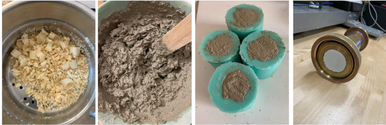
From Left to Right: Sifted 5mm Fibers, Concrete Paste, Molding of Samples, and Complete Sample in Impedance Tube
