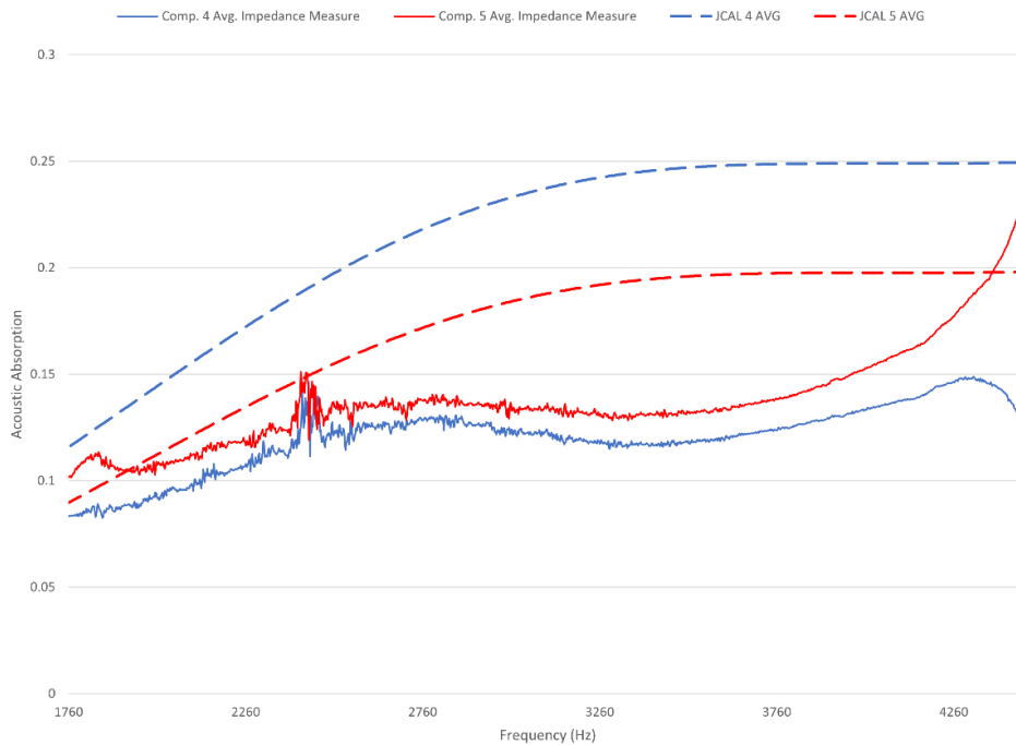
Figure 6-2: Comparison of Estimated and Measured Absorption of SD Concretes
