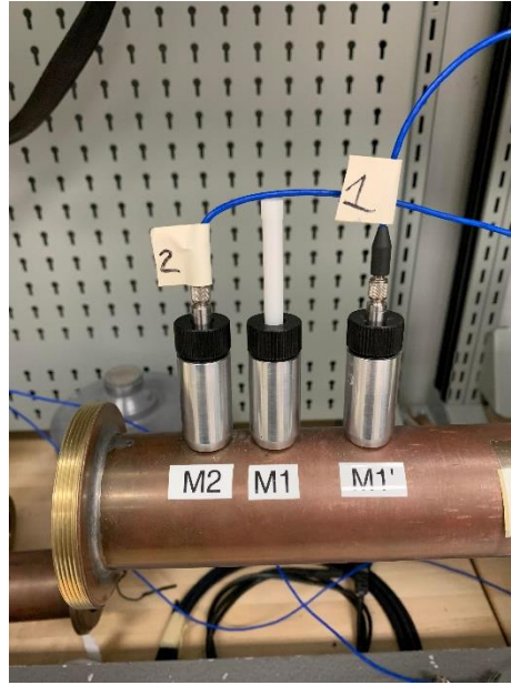
Figure 4-5: Microphone Positions on the Impedance Tube
