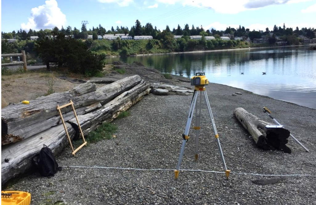
Figure 3 – Rotary laser level in place above a beach transect in Bremerton, Washington
