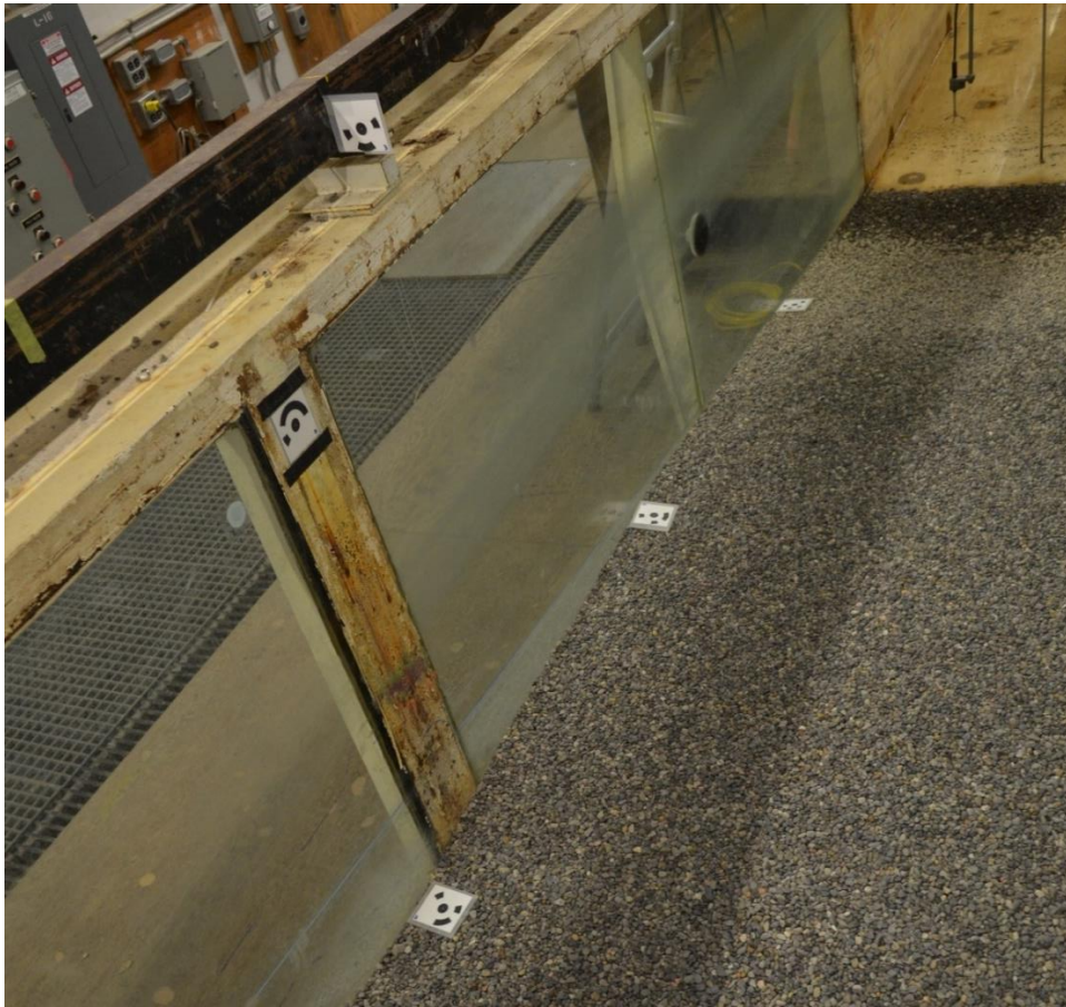
Figure 49 – Example of fixed markers attached to the flume's sidewall at known locations and mobile markers placed on the beach surface prior to taking photogrammetry photos
