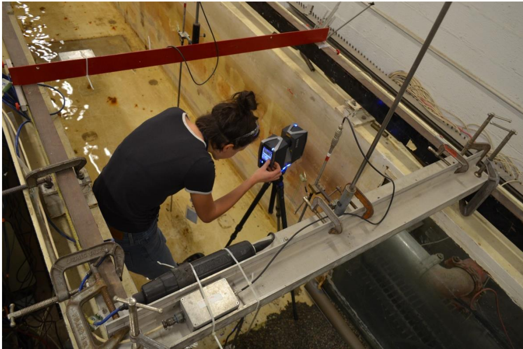
Figure 51 – FARO laser scanner set-up at the toe of the beach after draining the flume
