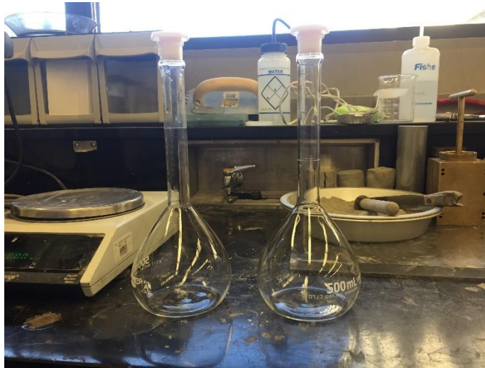
Figure 48 – Two pycnometers and hot plate used for Specific Gravity analysis
