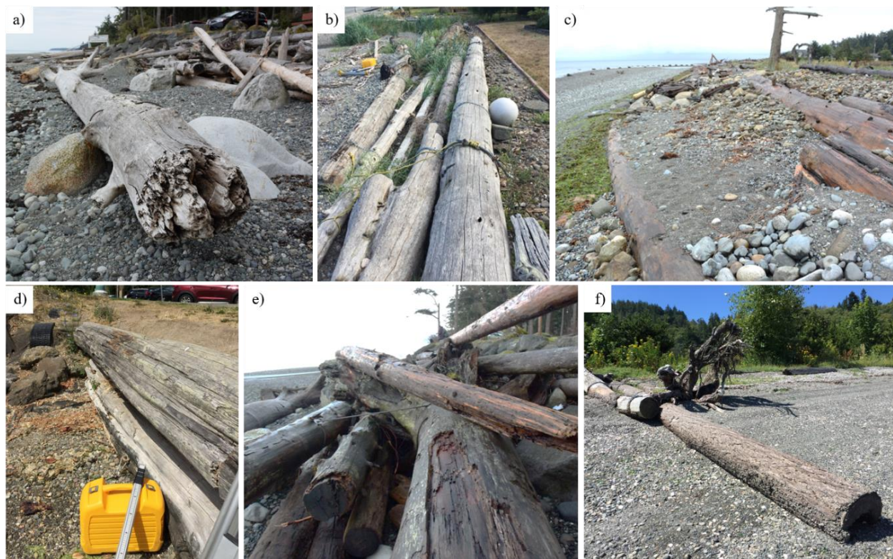
Figure 12 – LWD installation types observed during field surveys: (a) single, (b) multiple, (c) benched, (d) stacked, (e) matrix-style, or (f) groyne
