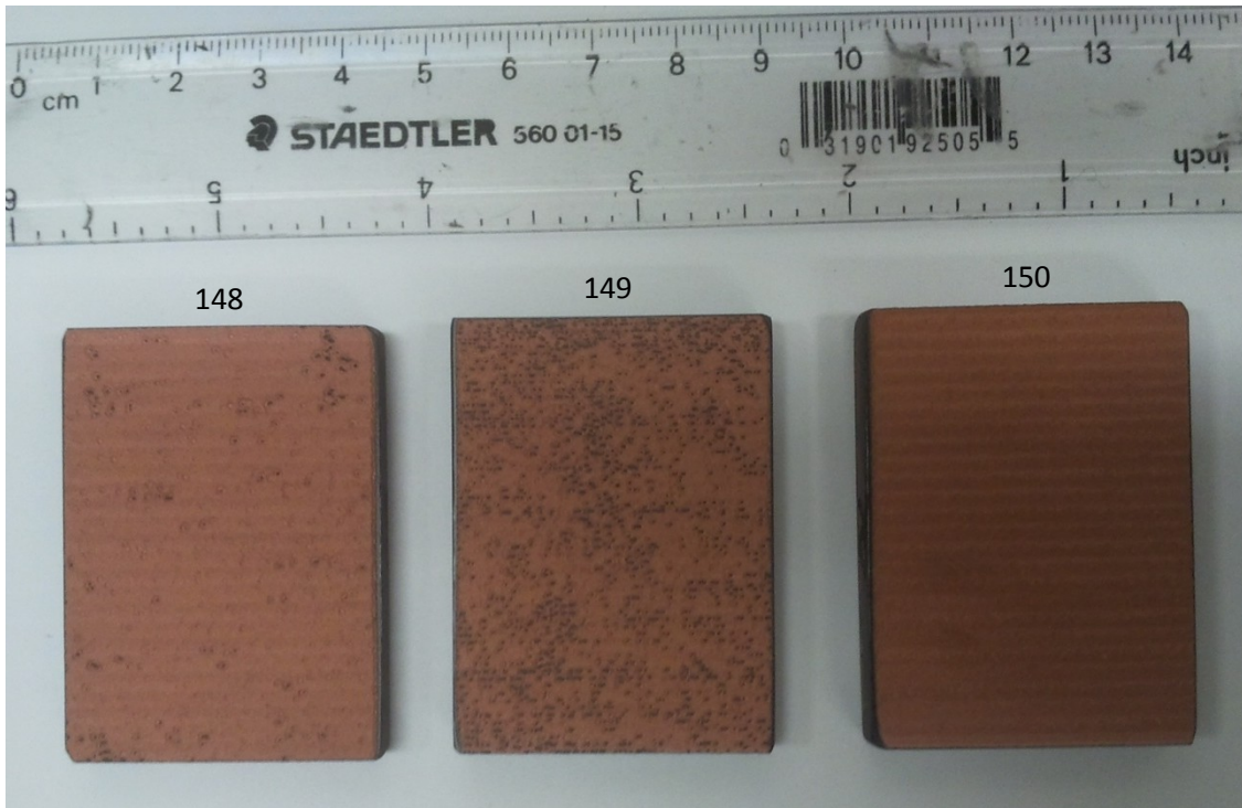
Figure 145: 97.5wt% SST-C5003 and 2.5wt% PEEK bond coat trial number 148, 149, and 150 on WGFP BMS 8-276.
