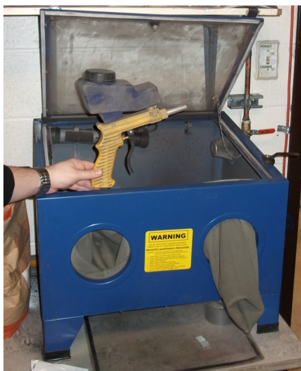
Figure 70: Grit blasting unit.
