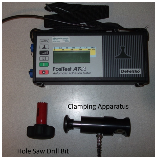
Figure 94: DeFelsko PosiTest AT-A adhesion testing apparatus.
