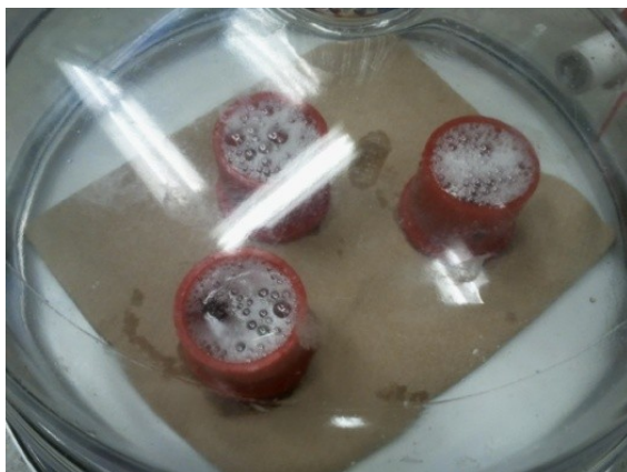
Figure 86: Resin filled moulds in glass bell vacuum chamber.
