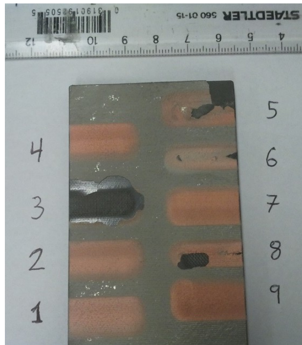
Figure 173: Pure copper (SST-C5003) top coat trials on tin (SST-S6001) coated WGFP BMS 8-276 composite.
