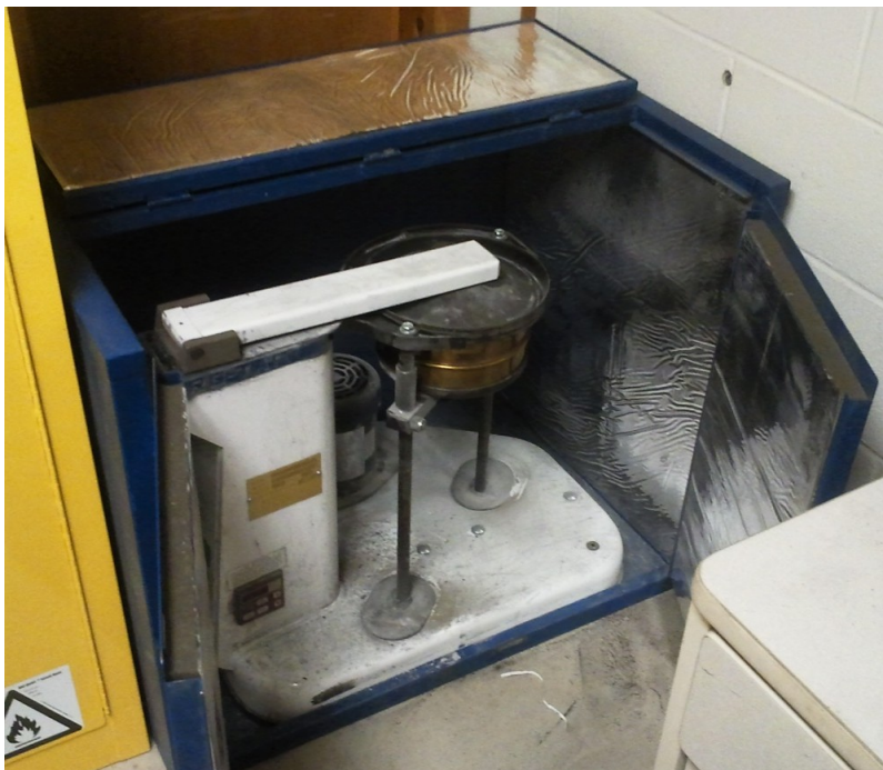
Figure 59: RX-29 sieve for W. S. Tyler.
