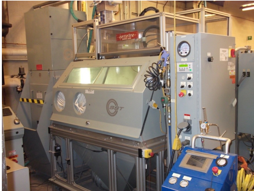
Figure 82: Centerline (Windsor) Ltd custom built spray chamber.
