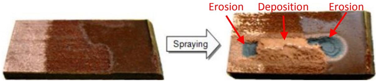
Figure 24: Effect of co-cured metallic bond coat finish on copper deposition (polished, unaltered rough, and resin rich) [29].
