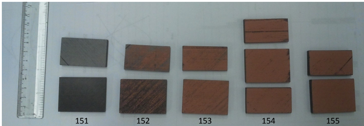
Figure 163: Deposited bond coats with varying feedstock composition.
