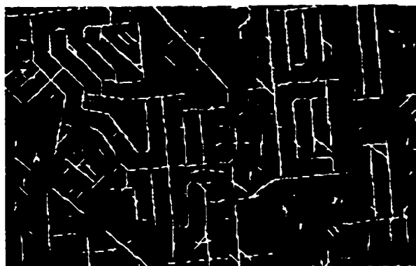
Figure 5.20: IMAGE 1 filtered with the parallel DRO filter with post-processing — \theta = 15, \theta_1 = 5, \theta_2 = 20
