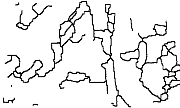
Figure 5.40: The parallel watershed transformation on IMAGE 2 with the marking function with n=2
