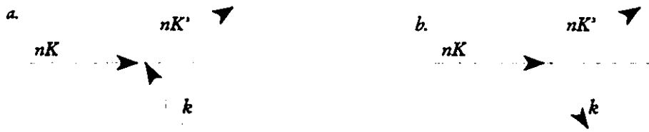
Figure 2.15 The scattering of a photon with a. absorption of a phonon (anti-Stokes) and b. emission of a phonon (Stokes). In both cases n is the refractive index of the material.
