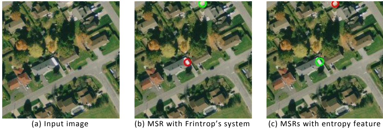
Figure 3-4: Red and green circles show the first and second MSRs respectively, when entropy is considered, or not, to measure saliency.
