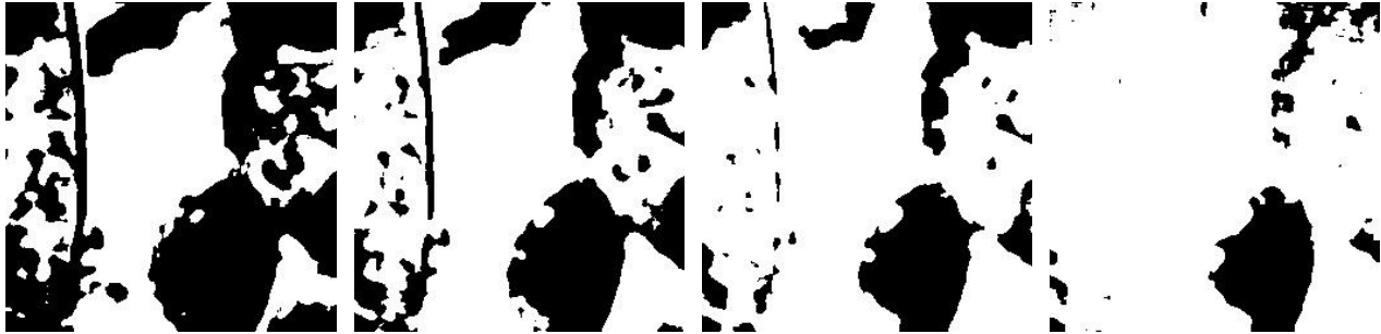
Figure 3-10: Variations in the detected region of interest as threshold values vary: from left to right T=1.5, 2.5, 3.5 and 5.0 .
