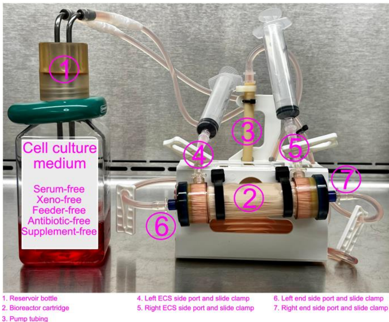
Figure 2: Hollow-Fiber Bioreactor (HFB) system component and set-up.
