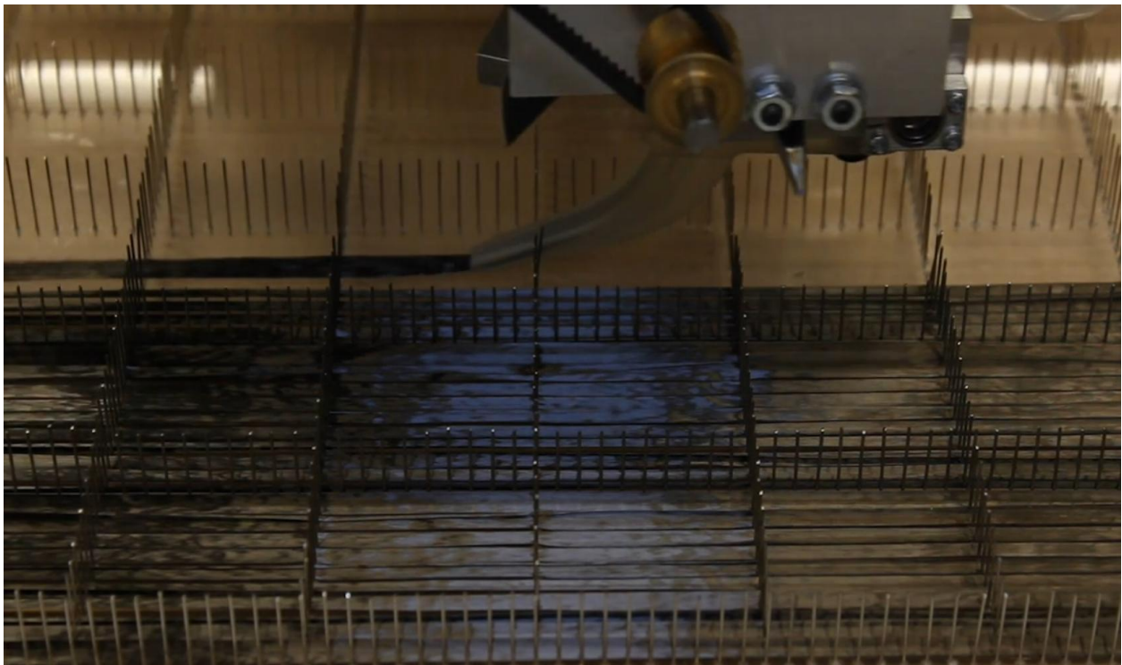
Figure 2-20: Carbon fibre yarn being laid between needle plate pins by YLM.
