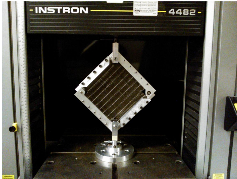
Figure 4-4: In-plane shear testing apparatus attached to 4482 Instron universal testing frame.
