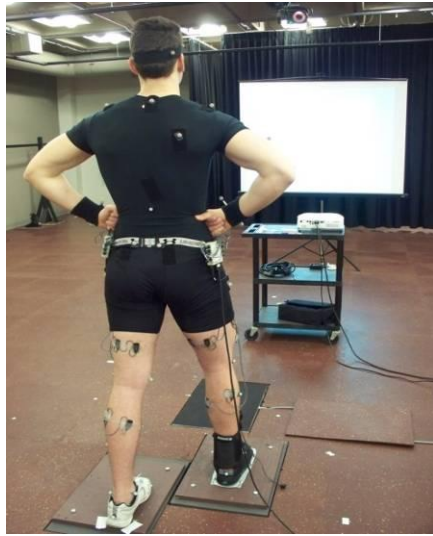
Figure 8: A) Laboratory setup B) Depiction of the target and cursor (Adapted from Williams et al., 2003). A successful match was achieved when the cursor was positioned over the target such that its circumference fits within the grey area of allowable error in the z-axis ( 50\% \text{ body weight} \pm 5\% ). Allowable error calculates to 3.9\% .
