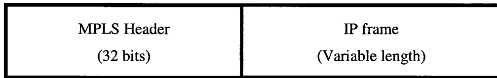
Figure 11. MPLS Header prepended to an IP Frame
