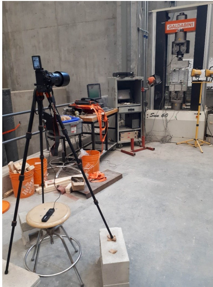
Figure 4.10: Reference camera mounted on a tripod and equipped with a long lens
