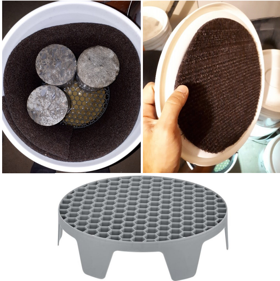
Figure 3.7: Conditioning of reactive cylinders inside 19L buckets with high humidity (> 95%) and temperature (38 °C)
