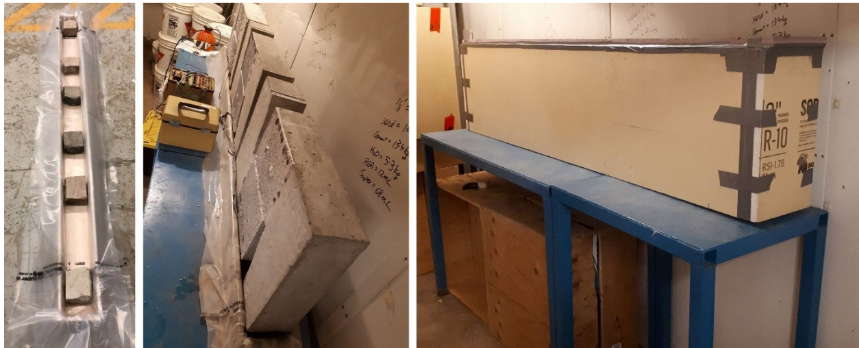
Figure 3.6: Conditioning of reactive push-off specimens inside a box with high humidity ( > 95\% ) and temperature ( 38\text{ }^{\circ}\text{C} )
