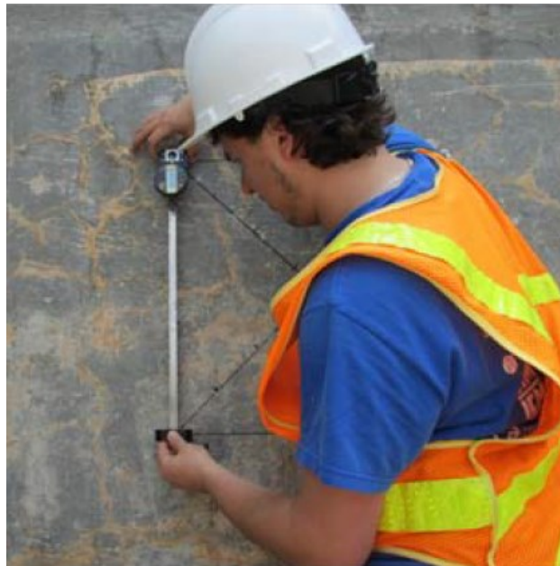
Figure 1.4: Expansion measurements using a DEMEC strain gauge (Thomas et al., 2013)
