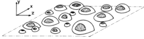
Figure 2.10: Contact areas during shear displacement (Walraven & Reinhardt, 1981)
