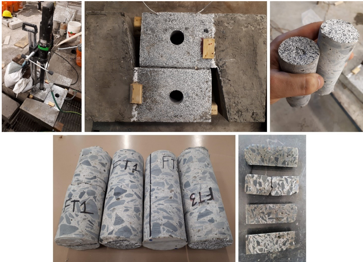
Figure 3.20: Coring of specimens 04I and 07I for petrographic analysis of ASR damage
