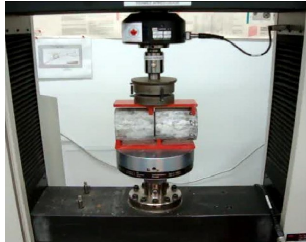
Figure 2.20: Cylindrical setup for testing the shear strength of concrete (Sanchez et al., 2016)
