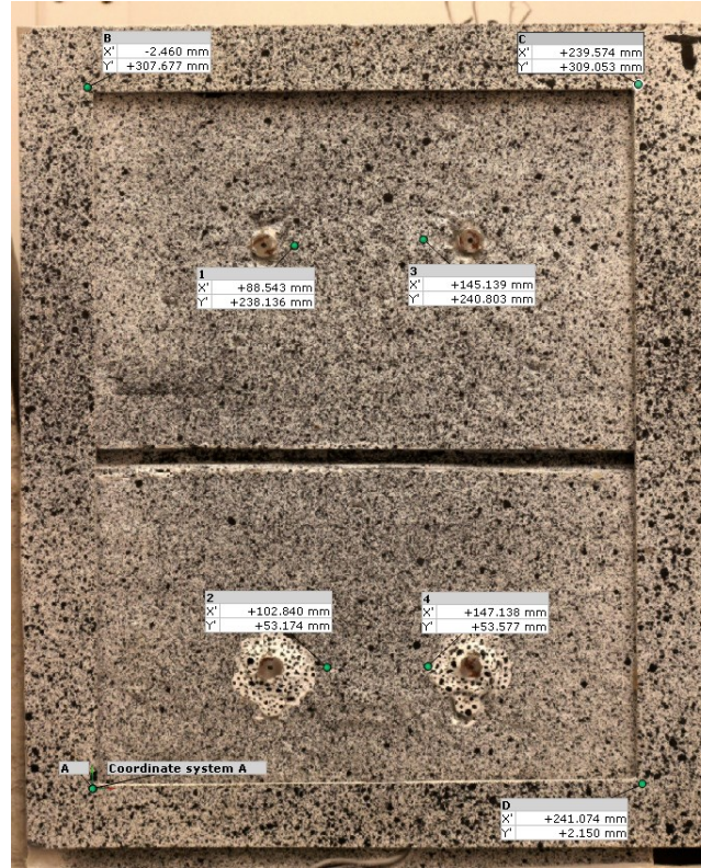
Figure 4.11: ASR expansion measurement with the correction method on GOM Correlate 2019
