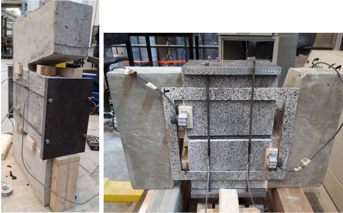
Figure 3.12: External prestressing apparatus
