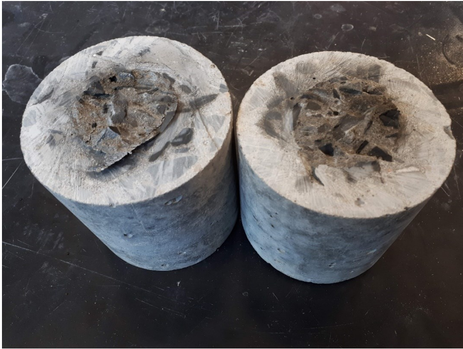
Figure 3.24: Cracked faces of companion cylinders tested under direct shear
