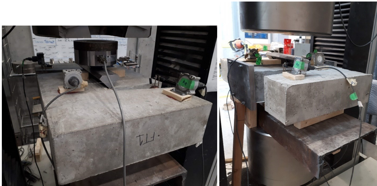
Figure 3.14: Pre-cracking phase before testing: internally reinforced specimen (left) and externally reinforced (right)
