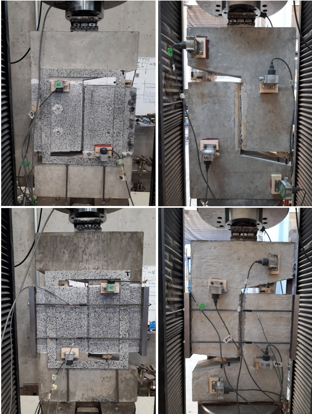
Figure 3.17: Internally reinforced (top) and externally reinforced (bottom) push-off specimens in the hydraulic testing machine: front view (left) and rear view (right)
