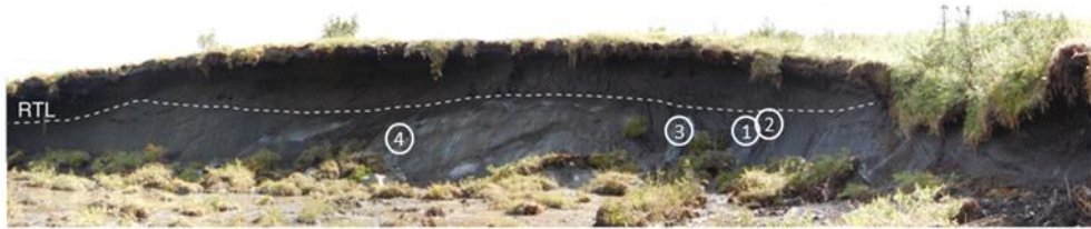
Fig. 4.2 Photograph of the headwall at Roger Thaw Slump, NWT, on August 1 st 2016, showing the four massive ice units, and the limit of the relict thaw layer (RTL) (RTS; 67°37'05.2"N, 135°33'23.2"W, 350 m a.s.l.).
