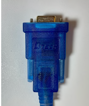
Figure 3.14 RS232c converter linked to the CyberTouch glove.
