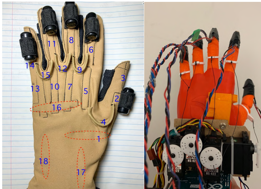
Figure 4.2 The back side view of the CyberTouch glove, and the Ring Ada robotic hand.
