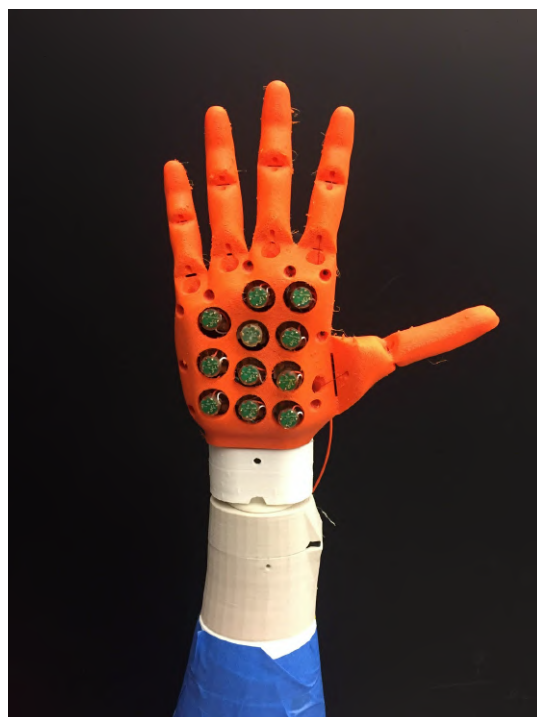
Figure 6.1 Prototype of multi-modal bio-inspired tactile sensor to equip Ada hand’s palm.
