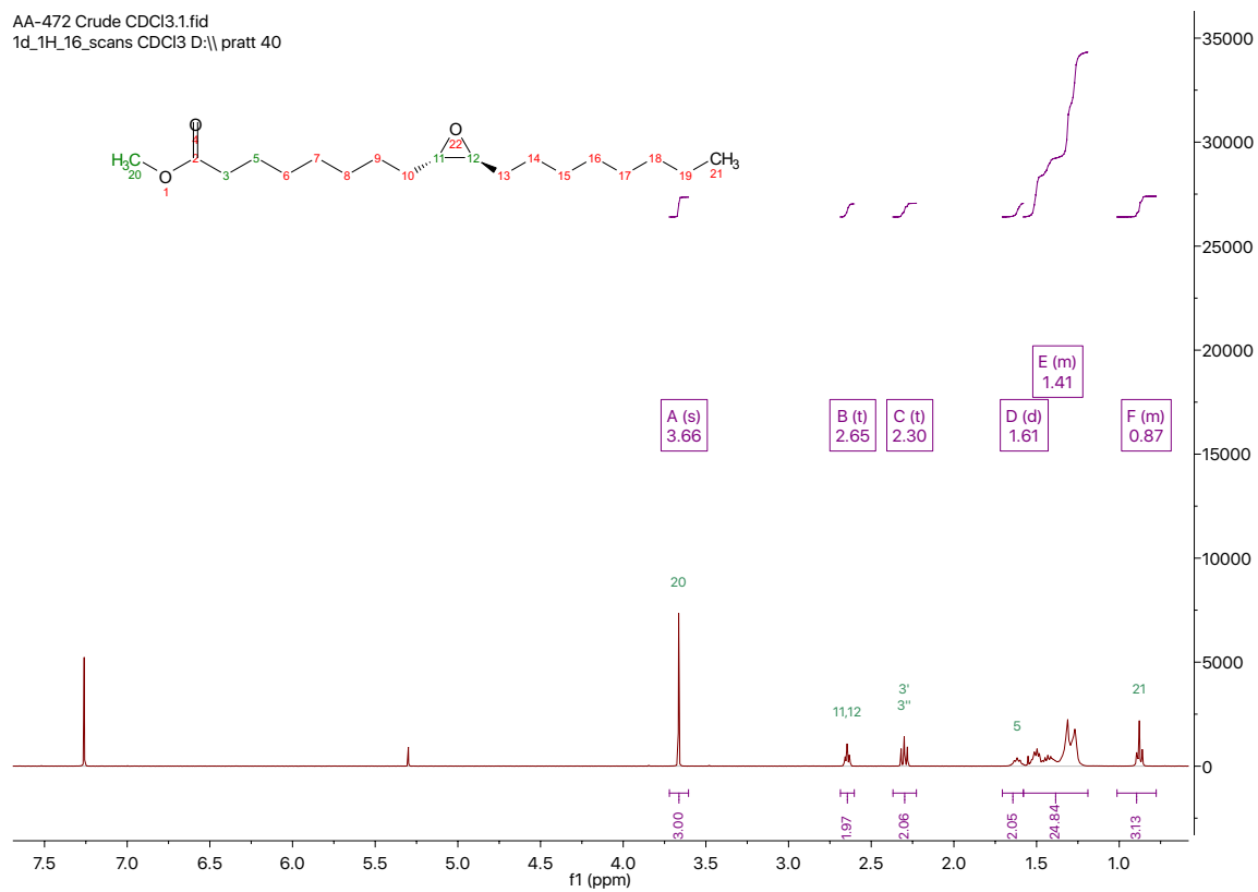
Figure 4.58 1 H NMR (CDCl 3 , 400 MHz) spectra of spectra of 9,10-trans-epoxide of methyl oleate (59).
