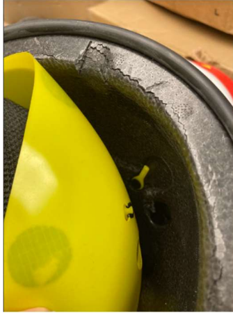
Figure 16. The suspension of the rotational technology broken between the liner and the shell of the helmet.
