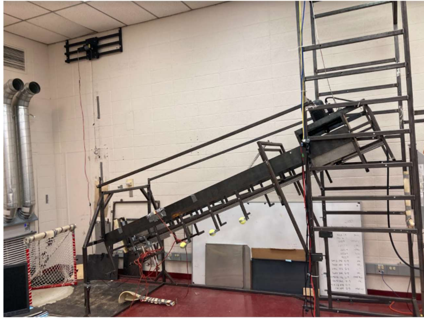
Figure 5. The rail guided launcher (RGL) used for all impacts.
