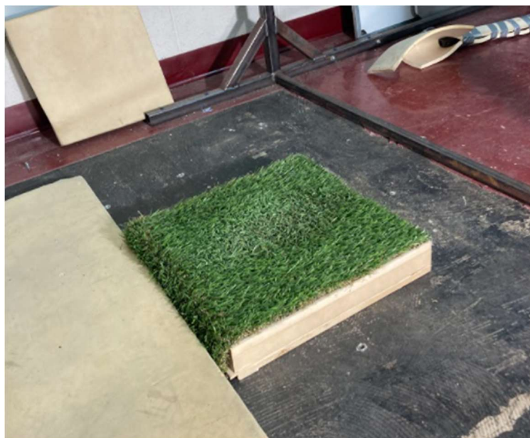
Figure 3. The high compliant anvil made of 66mm of 602 vinyl nitrile foam with synthetic foam on top.
