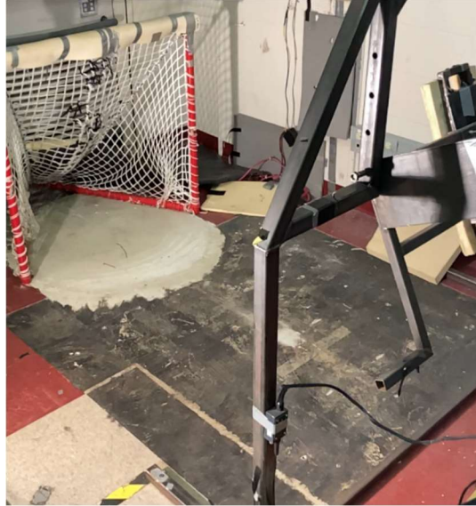
Figure 4a. The low compliant anvil that consisted of a bare concrete surface at the end of the rail guided launcher.
