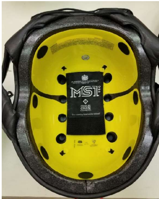
Figure 10. MS1 Pro Charles Owen equestrian helmet with MIPS technology and headband removed.
