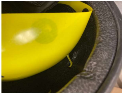
Figure 17. The suspension of the rotational technology connected between the liner and the shell of the helmet.
