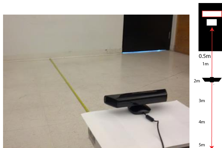
Figure 3.14 : Setup for experimental evaluation of sensitivity to color with respect to distance.
