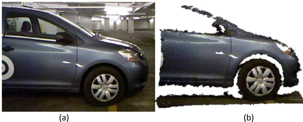
Figure 5.9 : Registration of color and depth images: a) color image, b) colored depth image.
