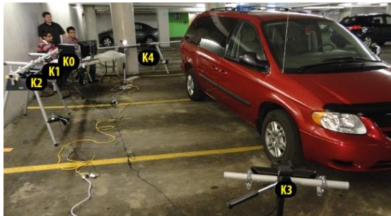
Figure 6.1 : Multi-camera acquisition platform setup in real operating environment.
