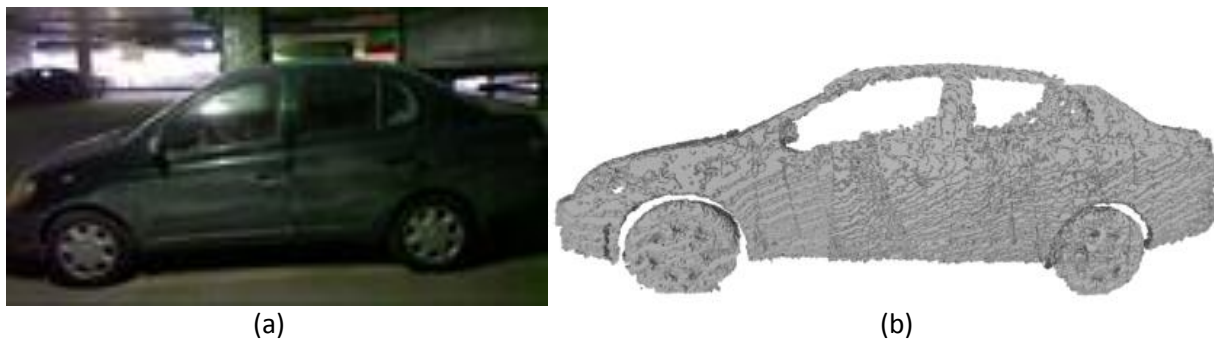
Figure 3.16 : Vehicle in a semi-outdoor parking garage: a) color image, b) 3D reconstruction.
