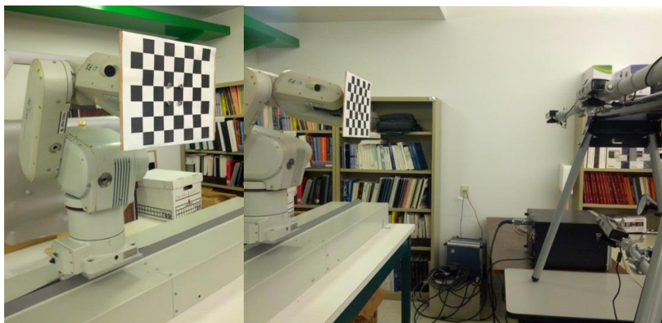
Figure 5.19 : Robot carrying a checkerboard target during vision-robot calibration.
