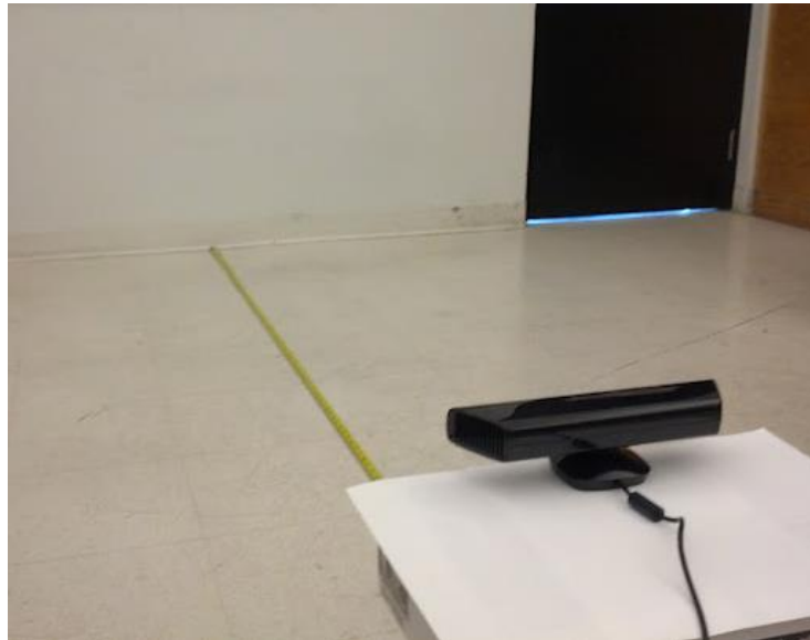
Figure 3.8 : Setup for experimental evaluation of depth estimation.
