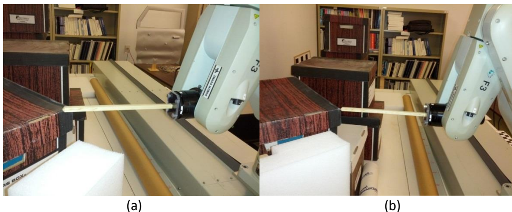
Figure 5.22 : Moving robot towards selected points with respect to robot base: a) reconstructed point b) exact point.
