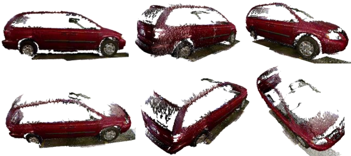
Figure 6.6 : Six different views of the reconstructed minivan.
