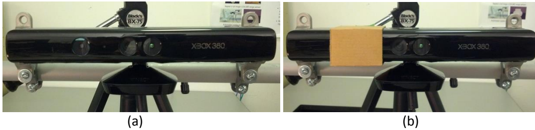
Figure 5.2 : Covering projector’s window during internal calibration: a) without mask b) with mask.
