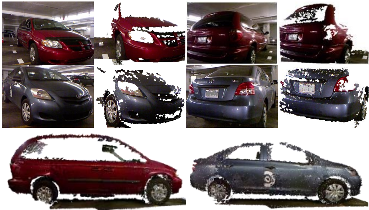
Figure 3.17 : Different views of a two vehicles and corresponding 3D reconstructions with missing depth areas depicted in white.
