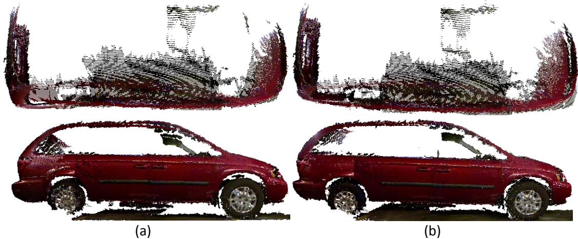
Figure 6.5 : Reconstruction of the vehicle using the proposed method a) without using ICP b) with ICP refinement.
