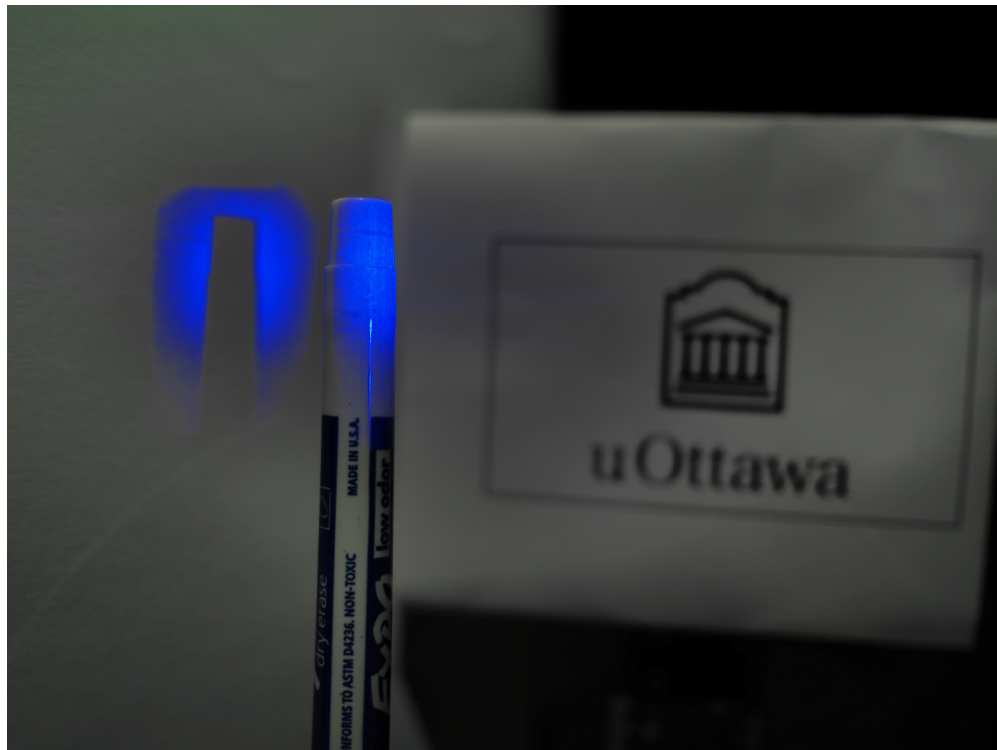
Figure 4.3: This figure had the same experimental setup as fig. 4.2, with the exception of the additional white light source illuminating from above. This allows the observation of the opaque object and Laser Shadow in context. Due to the depth of field of the image, the Laser Shadow is visible in the foreground on the opaque object. The background is out of focus, which makes the observation of the Laser Shadow difficult from this figure.
