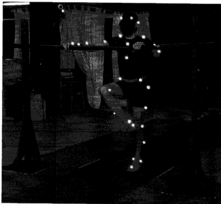
Figure A 1. Instrumented participant performing dynamic ROM trial (external rotation at 90° of hip flexion) while holding on to support frame.
