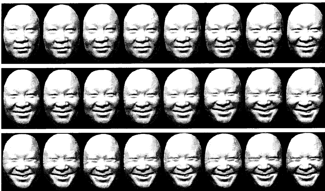
Figure 7-9 Sequence of measurement result of human facial expressions with the six-step triangular-pattern phase-shifting method. The triangular pattern were generated with a pitch of 18 pixels.
