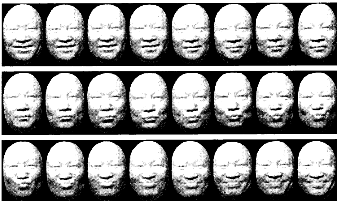
Figure 7-8 Sequence of measurement results of human facial expressions with the five-step triangular-pattern phase-shifting method. The triangular patterns were generated with a pitch of 20 pixels.
