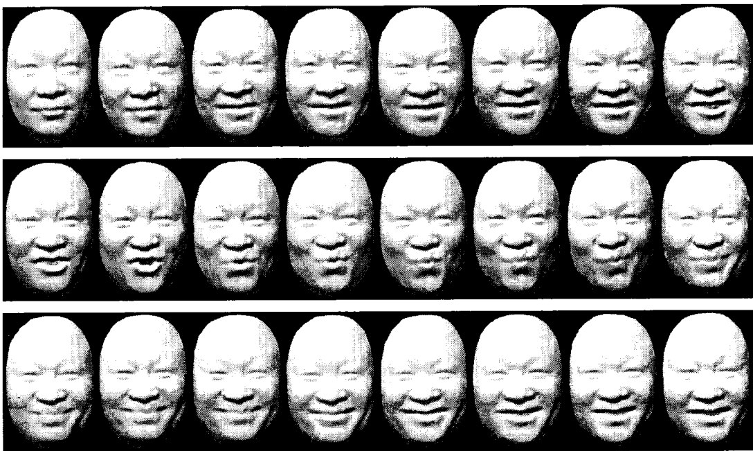
Figure 7-7 Sequence of measurement results of human facial expressions with the four-step triangular-pattern phase-shifting method. The triangular patterns were generated with a pitch of 16 pixels.
