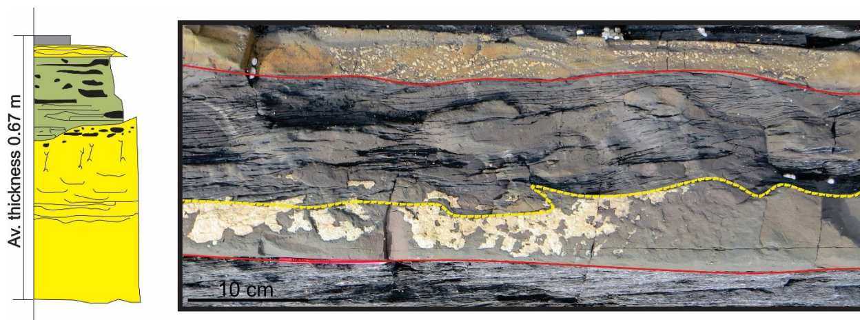
Figure 39. Schematic of a linked debrite (redrawn from Haughton et al., 2003) and representative photograph from the Ordovician Cloridorme Formation (Quebec, Canada); red lines indicate bed bases and dashed yellow line indicates the contact between the lower turbidite and upper debrite.
