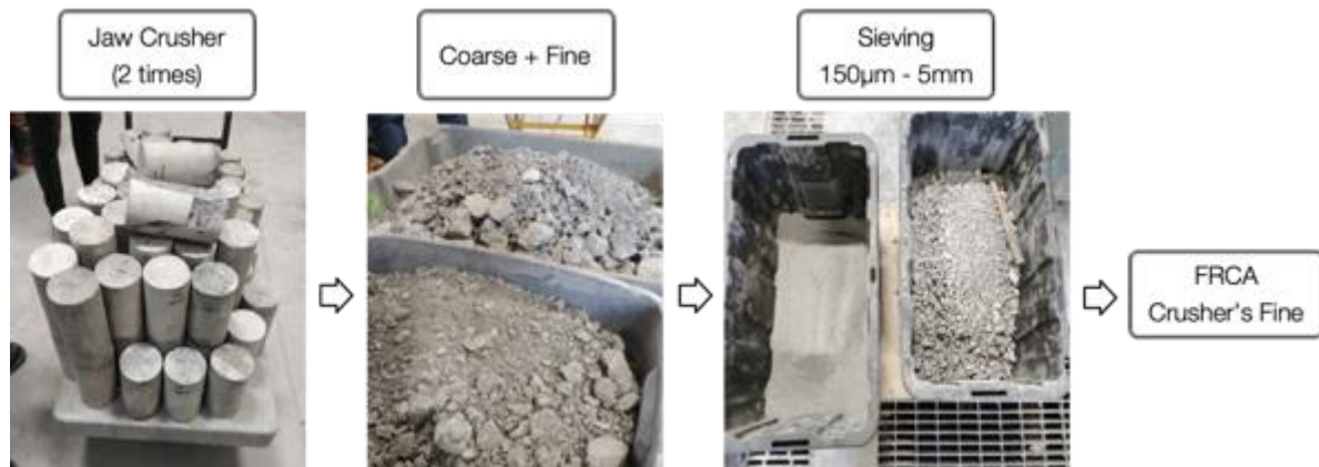
Figure 3.2: Summary of first method of production (CF) where both coarse and fine fractions are produced.
