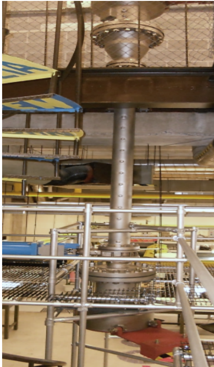
Figure A-1. High-pressure fluidization column
