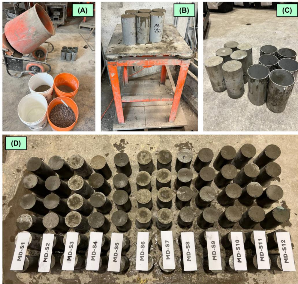
Figure 5.7: Making cylinders for the second phase of the experimental program; (A) Mixing the materials, (B) Vibration, (C) Opening the molds, and (D) All seventy-two cylinders
