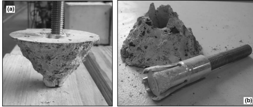
Figure 2.3: Pull-out test on concrete (Brencich et al., 2021)
