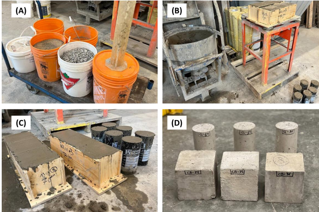
Figure 3.7: The casting of cubic and cylindrical specimens in the laboratory; (A) materials, (B) mixing and vibrating, (C) molds, and (D) specimens
