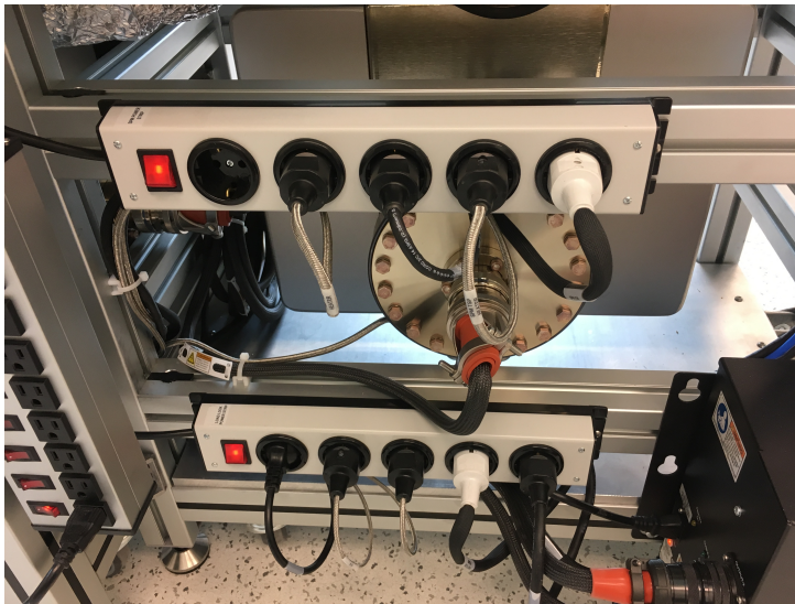
Figure 3: SPM (top) and Load lock (bottom) power strips. The plugs run through those listed in Step 11 from left to right.
