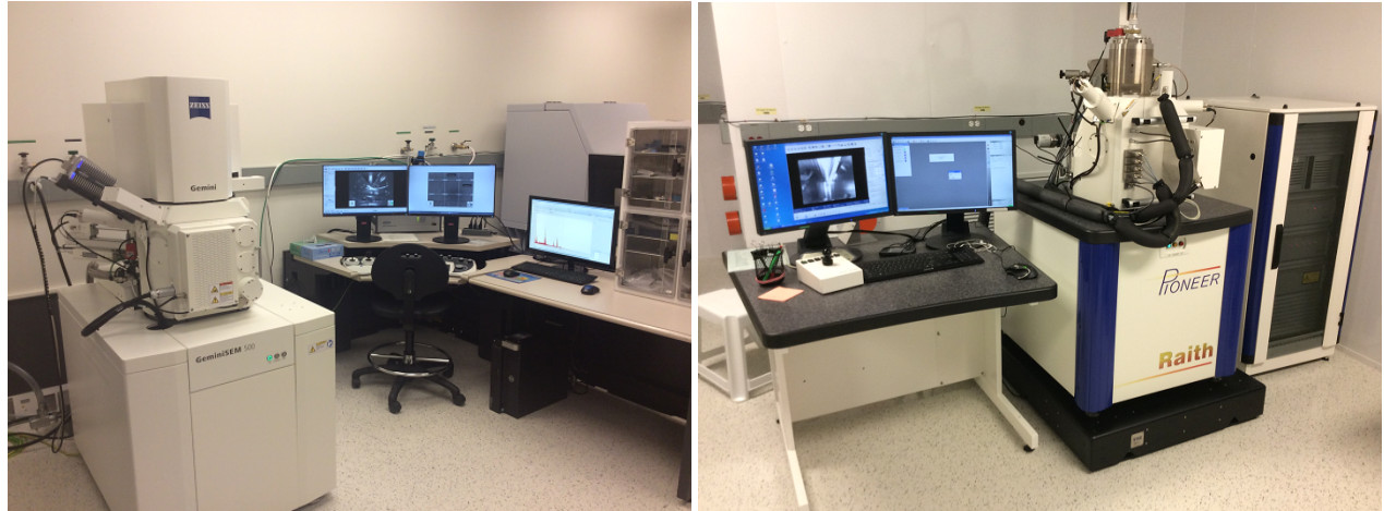
Figure 8.9: Scanning electron microscopes used for characterization and electron-beam lithography. (a) Gemini 500 SEM. (b) Raith Pioneer.
