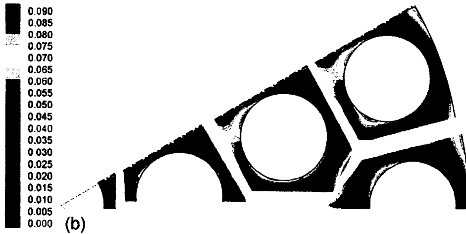
Figure 9 - 4 (a) Dimensionless standard deviation of radial velocity fluctuations u'_r / \bar{U}_{\max} around the middle outer rod ; — simulations ; \circ OT experiments ; (b) predicted isocontours of u'_r / U_b in local coordinates
