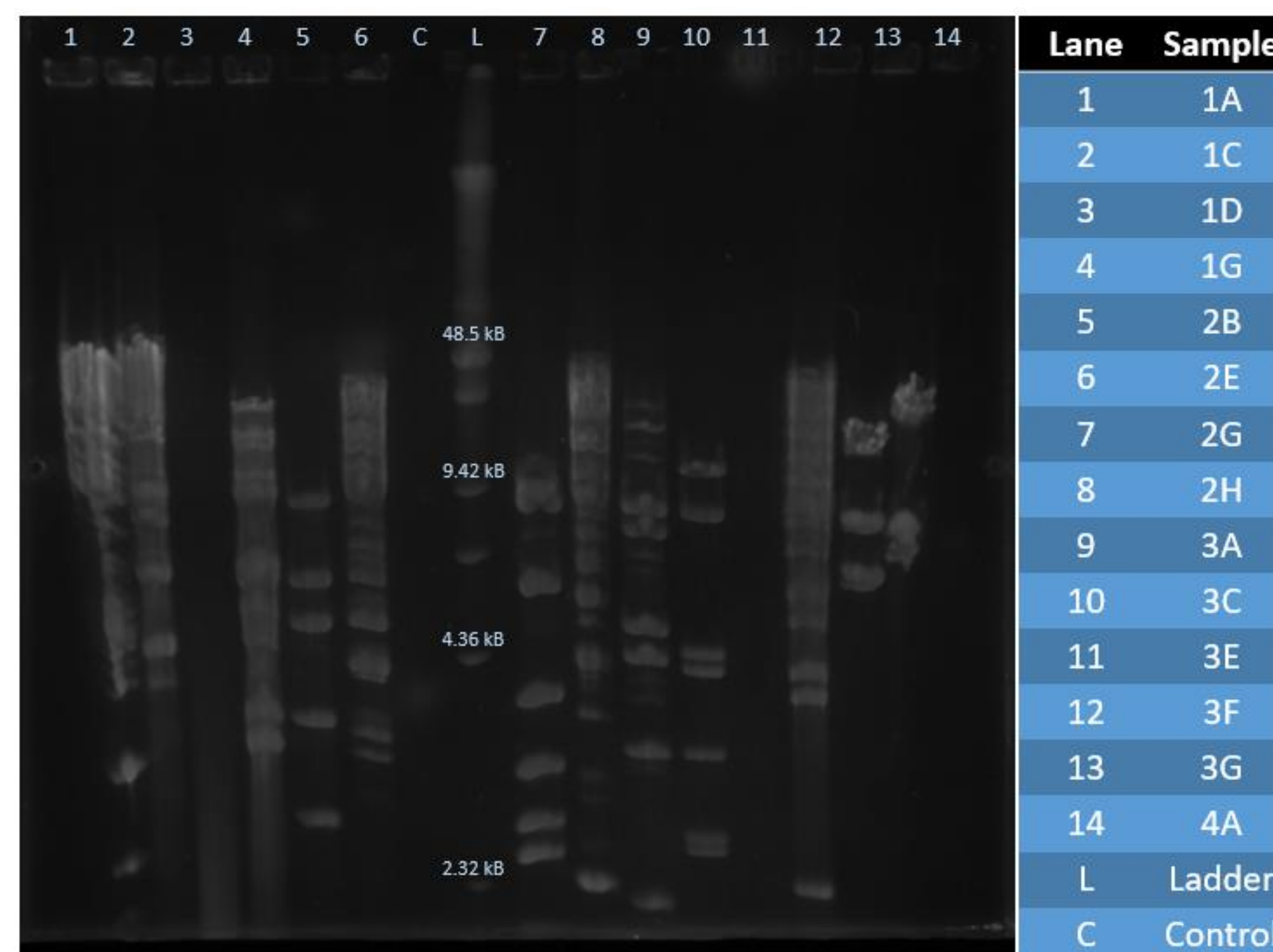
Figure 2. Pulse field gel electrophoresis. 14 extracted samples were digested with HindIII and BamHI, gel was run for 24 hours at 145 V. Backbone 8.1 kb, insert up to 42 kb.
