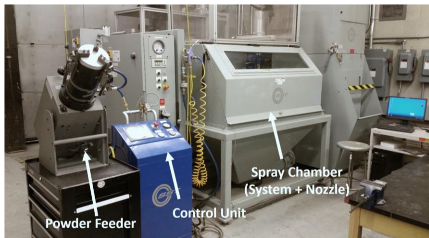
Figure 53 - Cold spray system used for all experiments
