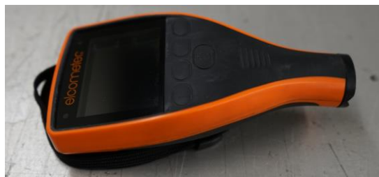
Figure 52 - Coating thickness measurement instrument: Elcometer®
