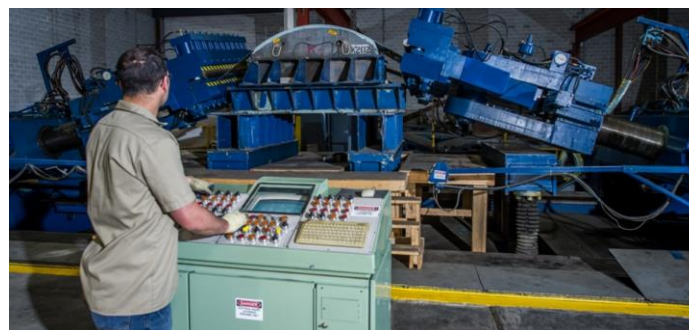
Figure 6 - Process of stretch-forming [33]
