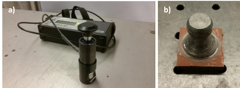
Figure 58 - Image of: a) PATTI, b) dolly glued and secured on copper coated CFRC
