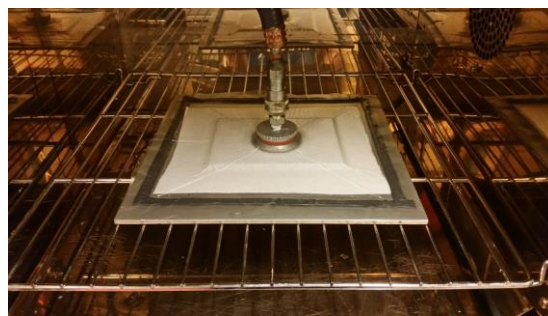
Figure 57 - Vacuum bagged assembly in controlled convection oven
