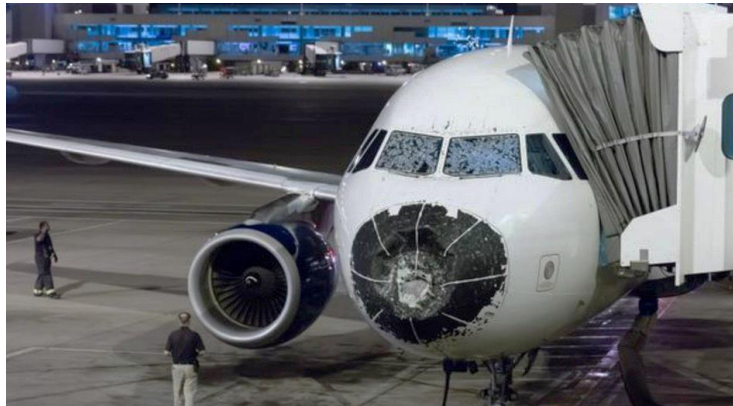
Figure 4 - Image of Delta Air Lines Flight 1889, erosion damage by hailstones [31]
