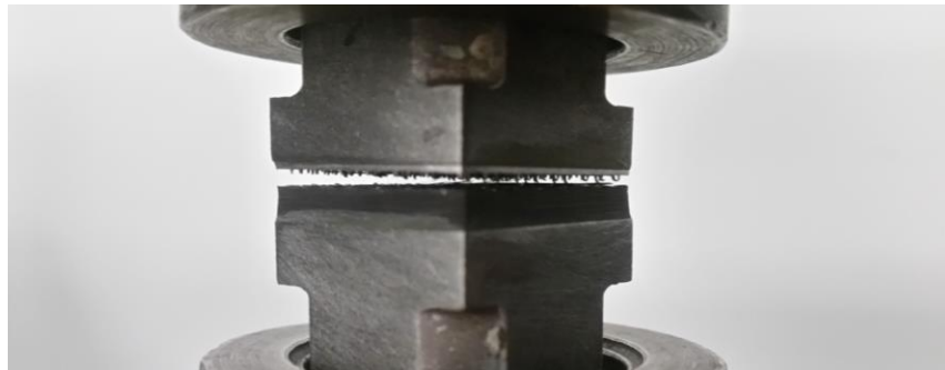
Figure 119 - Phase 2: Example of GRIP Metal™-CFRC after failure
