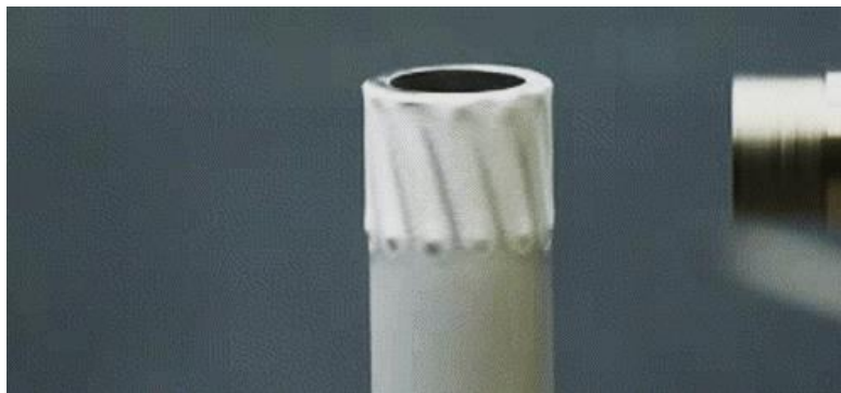
Figure 26 - Cold spray gear teeth on shaft [53]
