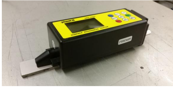
Figure 51 - Profilometer on top of an Invar sample
