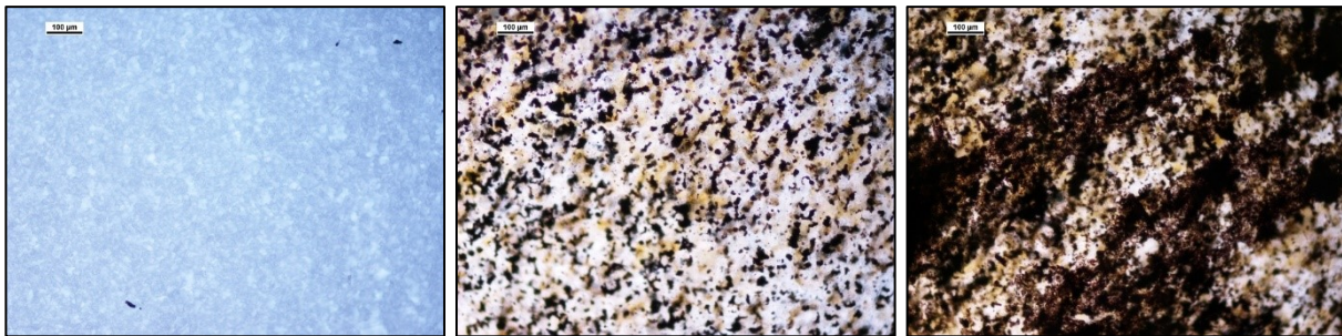
Figure A. 18: Optical microscope image of 5 µm PTFE membrane at 100x magnification before (left) and after bio-oil microfiltration (middle and right) showing different levels of fouling on surface of membrane
