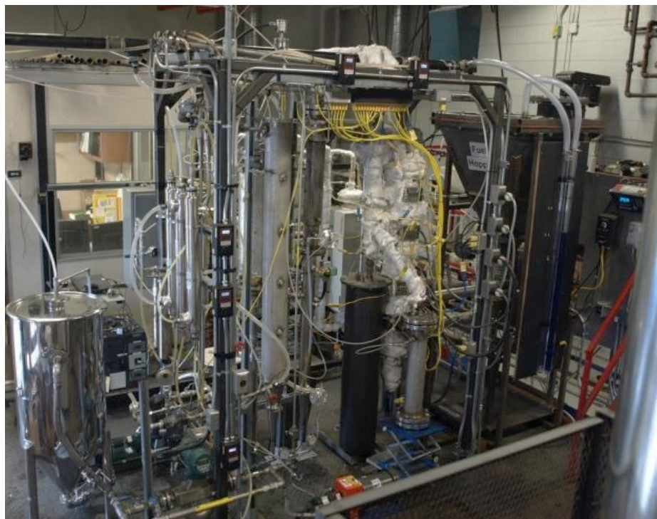
Figure A. 8: Image of CanmetENERGY-Ottawa's 5-10 kg h -1 bubbling bed fluidized fast pyrolysis system
