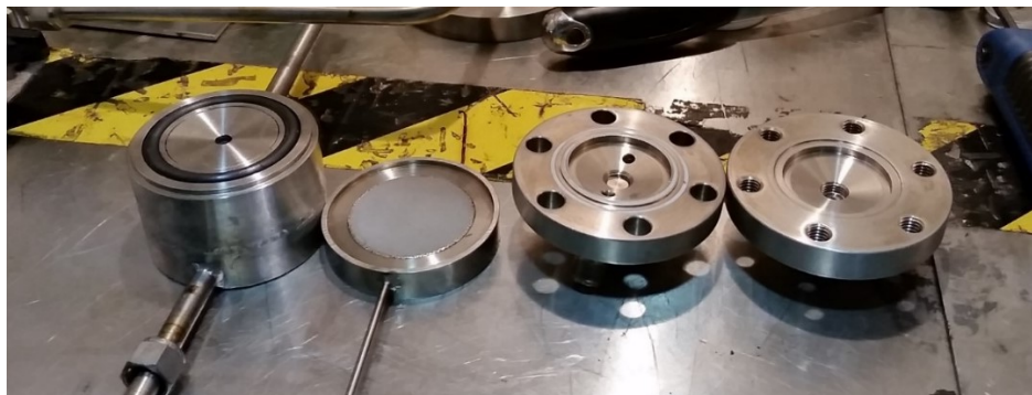
Figure A. 4: Filtration cells used in early proof-of-concept experimental trials with the MRK 1 microfiltration system; disassembled cell 1 on the left, disassembled cell 2 on the right
