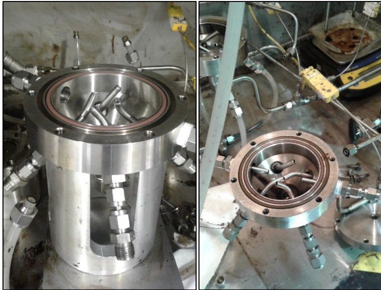
Figure A. 5: Side view of different flow configurations for prototype filtration cell used in bio-oil microfiltration studies with the MRK II and MRK III experimental system
