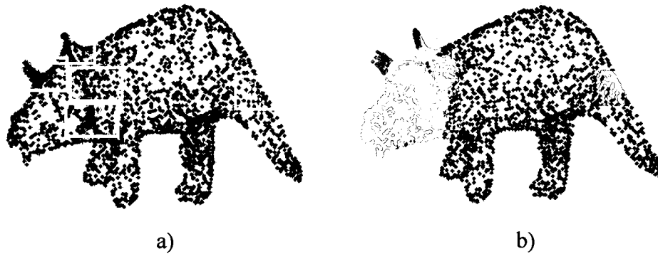
Fig. 5.34. (a) Areas of elasticity change detected in the growing neural gas map and (b) the corresponding selectively densified point-cloud.
