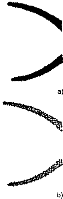
Fig. 4.16. Pliers model with non-homogeneous compliance, without significant localized changes in compliance (a) point-cloud and (b) neural gas model with compliance for a map of 20×25.
