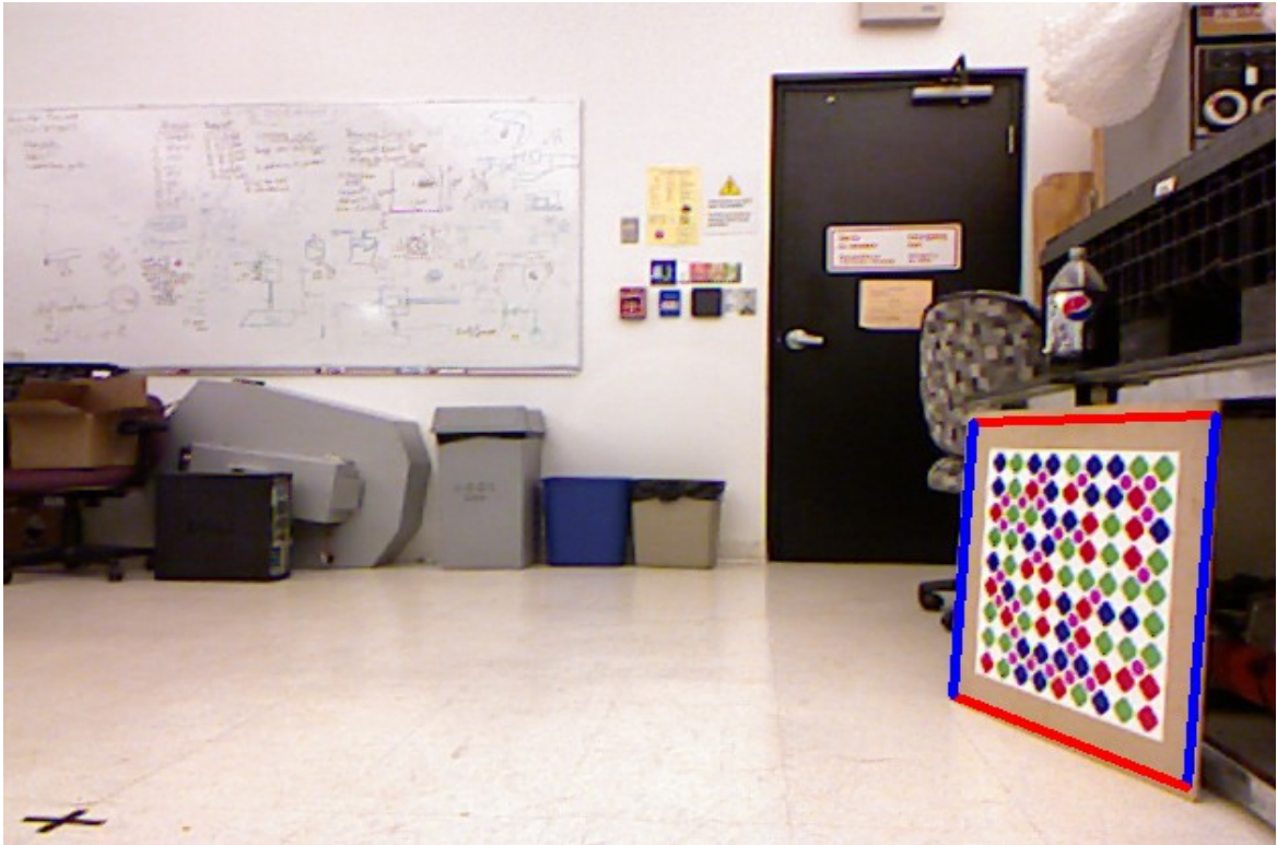
Figure 1.1: Sample image of marker detection. Detection of the proposed marker system used to navigate an autonomous robot within an office laboratory environment.
