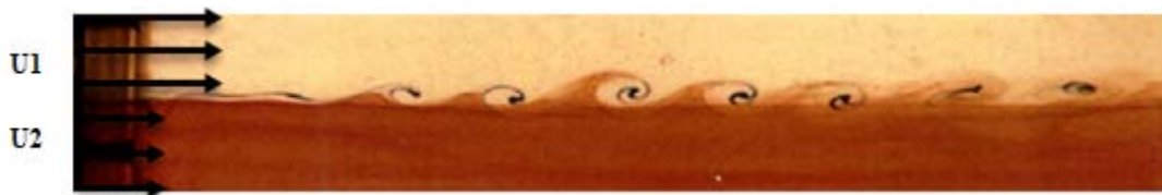
Fig. 1: Streamwise evolution of a 2D mixing layer behind the flat plate - vortex rollup (Lasheras and Choi, 1988)
