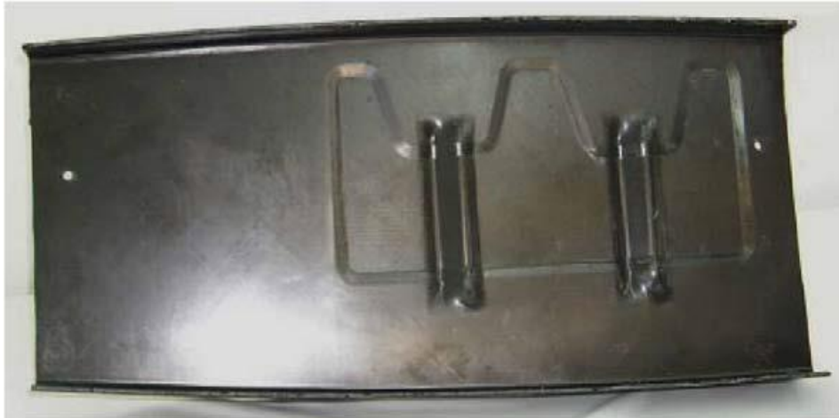
Figure 1.3. Aircraft wing rib element produced by RTM [6]
