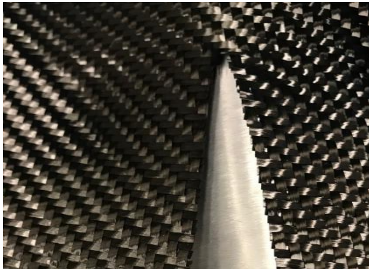
Figure 7.2. Fraying around edges after cutting and draping, carbon fibre fabric 104
