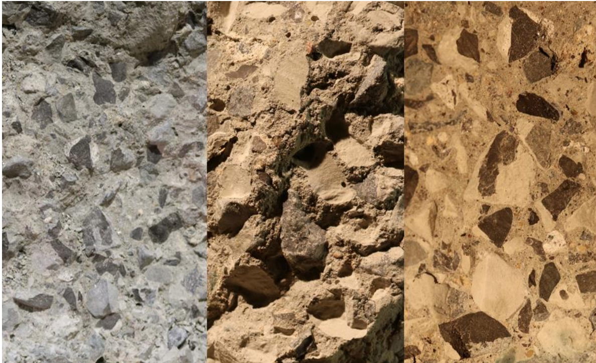
From left to right: photos of shear failure planes for control, 50% RCA and 100% RCA beams
